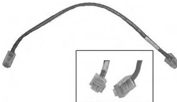
Figure 9.5 Ethernet crossover cables.
