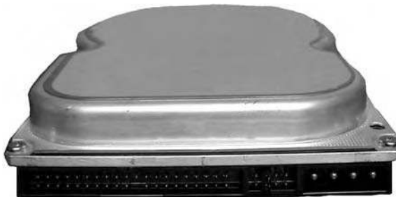
Figure 4.10 Hard drive—back view.
