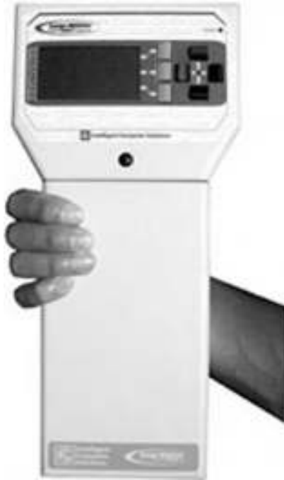
Figure 3.4 ICS Image MASSter Solo 2 hand-held forensic unit (Reprinted with permission, 2002.)
