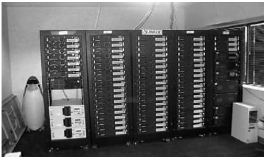
Figure 3.3 A forensic Linux Beowulf cluster.
