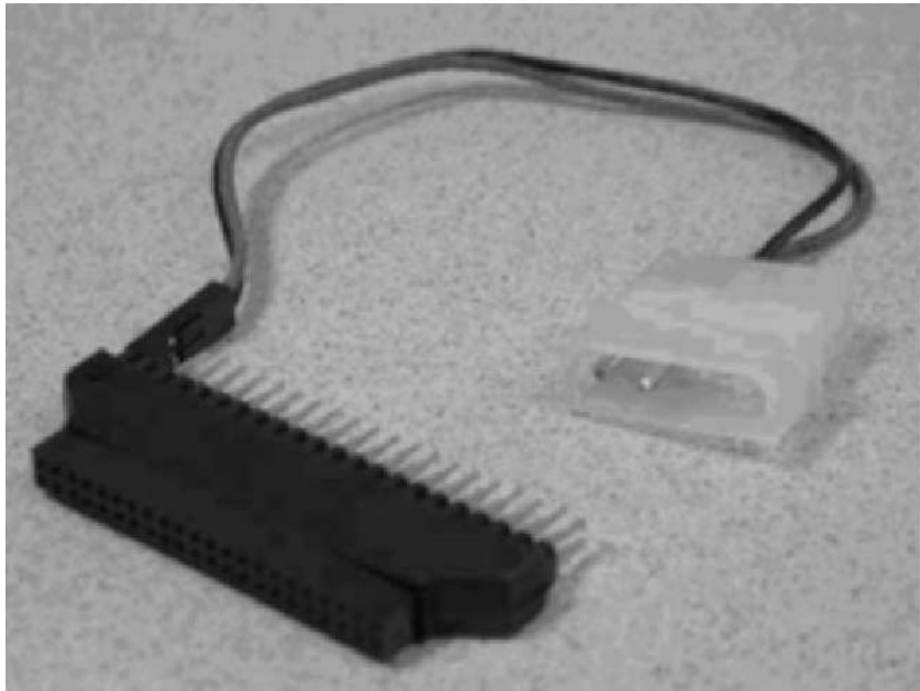
Figure 4.1 A 2.5" to 3.5" PATA IDE Conversion Cable
