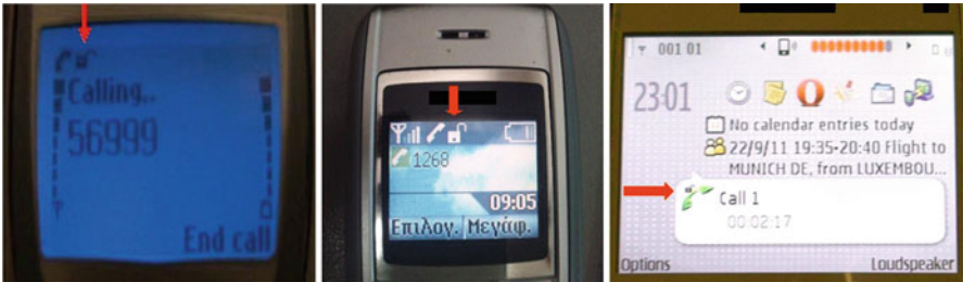
Fig. 3.9 The unlocked padlock indicates (a little more descriptively) the lack of encryption
