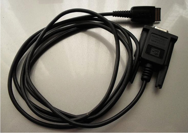
Fig. 4.6 Serial port cable for connecting the phone to PC and issuing of AT commands
