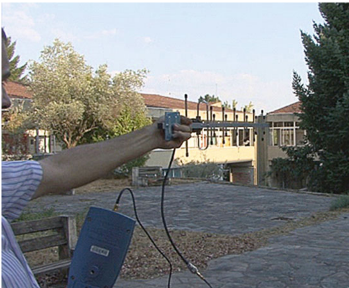
Fig. 1.3 Directional antenna locating mobile phone transmissions (after [44])
