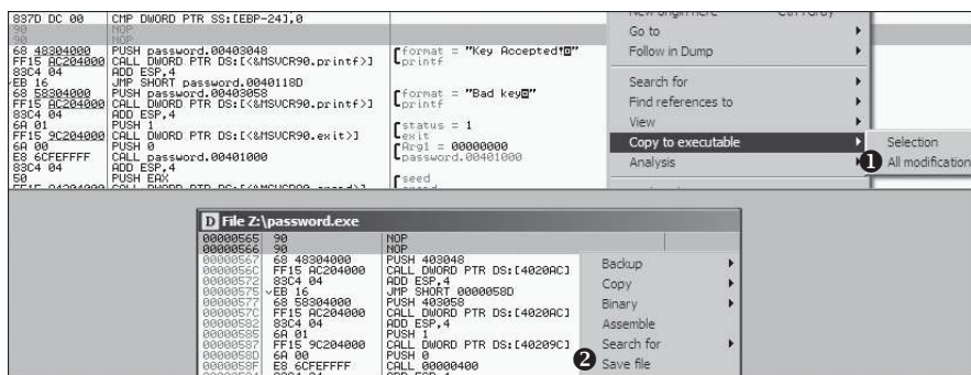
Figure 9-14: Two-step process for copying a live memory patch to an executable on disk
