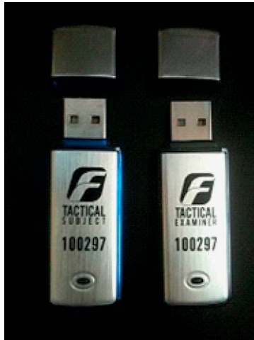
FIGURE 1.64 —The F-Response TACTICAL “Subject” and “Examiner” dongles.
