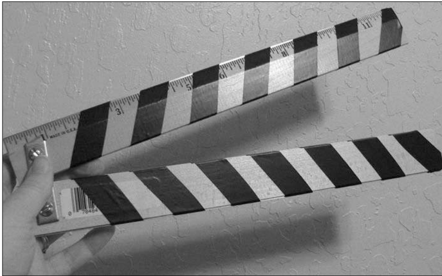
Figure 11-3: Make yourself a clapstick, or use a commercially available clapstick slate, when recording audio separately from the video.
