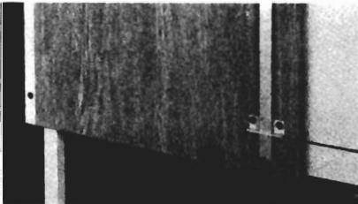
RETAINER CLIP HOLDING DOOR AGAINST CABINET
