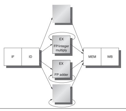
**Figure C.33** The MIPS pipeline with three additional unpipelined, floating-point, functional units. Because only one instruction issues on every clock cycle, all instructions go through the standard pipeline for integer operations. The FP operations simply loop when they reach the EX stage. After they have finished the EX stage, they proceed to MEM and WB to complete execution.
