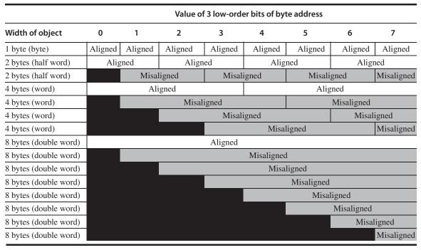
**Figure A.5** Aligned and misaligned addresses of byte, half-word, word, and double-word objects for byte-addressed computers. For each misaligned example some objects require two memory accesses to complete. Every aligned object can always complete in one memory access, as long as the memory is as wide as the object. The figure shows the memory organized as 8 bytes wide. The byte offsets that label the columns specify the low-order 3 bits of the address.
