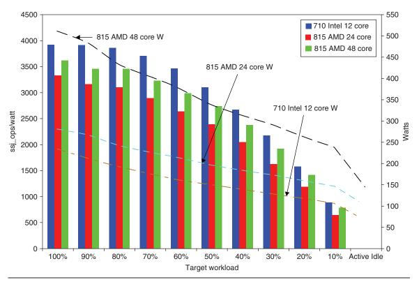
**Figure 1.19** Power-performance of the three servers in Figure 1.18. Ssj\_ops/watt values are on the left axis, with the three columns associated with it, and watts are on the right axis, with the three lines associated with it. The horizontal axis shows the target workload, as it varies from 100% to Active Idle. The Intel-based R715 has the best ssj\_ops/watt at each workload level, and it also consumes the lowest power at each level.
