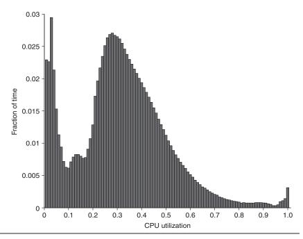
**Figure 6.3** Average CPU utilization of more than 5000 servers during a 6-month period at Google. Servers are rarely completely idle or fully utilized, instead operating most of the time at between 10% and 50% of their maximum utilization. (From Figure 1 in Barroso and Hölzle [2007].) The column the third from the right in Figure 6.4 calculates percentages plus or minus 5% to come up with the weightings; thus, 1.2% for the 90% row means that 1.2% of servers were between 85% and 95% utilized.
