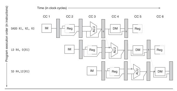
**Figure C.8** Forwarding of operand required by stores during MEM. The result of the load is forwarded from the memory output to the memory input to be stored. In addition, the ALU output is forwarded to the ALU input for the address calculation of both the load and the store (this is no different than forwarding to another ALU operation). If the store depended on an immediately preceding ALU operation (not shown above), the result would need to be forwarded to prevent a stall.
