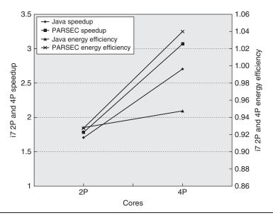
**Figure 5.30** This chart shows the speedup for two- and four-core executions of the parallel Java and PARSEC workloads without SMT. These data were collected by Esmaeilzadeh et al. [2011] using the same setup as described in Chapter 3. Turbo Boost is turned off. The speedup and energy efficiency are summarized using harmonic mean, implying a workload where the total time spent running each 2p benchmark is equivalent.
