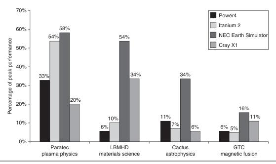
**Figure 1.20** Percentage of peak performance for four programs on four multiprocessors scaled to 64 processors. The Earth Simulator and X1 are vector processors (see Chapter 4 and Appendix G). Not only did they deliver a higher fraction of peak performance, but they also had the highest peak performance and the lowest clock rates. Except for the Paratec program, the Power 4 and Itanium 2 systems delivered between 5% and 10% of their peak. From Oliker et al. [2004].
