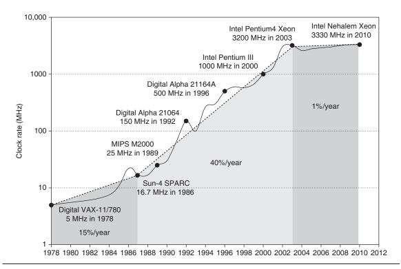
**Figure 1.11** Growth in clock rate of microprocessors in Figure 1.1. Between 1978 and 1986, the clock rate improved less than 15% per year while performance improved by 25% per year. During the "renaissance period" of 52% performance improvement per year between 1986 and 2003, clock rates shot up almost 40% per year. Since then, the clock rate has been nearly flat, growing at less than 1% per year, while single processor performance improved at less than 22% per year.
