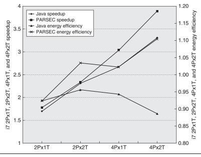
**Figure 5.31** This chart shows the speedup for two- and four-core executions of the parallel Java and PARSEC workloads both with and without SMT. Remember that the results above vary in the number of threads from two to eight, and reflect both architectural effects and application characteristics. Harmonic mean is used to summarize results, as discussed in the caption of Figure 5.30.
