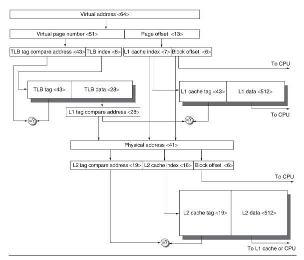
**Figure B.25** The overall picture of a hypothetical memory hierarchy going from virtual address to L2 cache access. The page size is 8 KB. The TLB is direct mapped with 256 entries. The L1 cache is a direct-mapped 8 KB, and the L2 cache is a direct-mapped 4 MB. Both use 64-byte blocks. The virtual address is 64 bits and the physical address is 41 bits. The primary difference between this simple figure and a real cache is replication of pieces of this figure.
