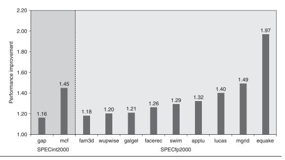
**Figure 2.10** Speedup due to hardware prefetching on Intel Pentium 4 with hardware prefetching turned on for 2 of 12 SPECint2000 benchmarks and 9 of 14 SPECfp2000 benchmarks. Only the programs that benefit the most from prefetching are shown; prefetching speeds up the missing 15 SPEC benchmarks by less than 15% [Singhal 2004].
