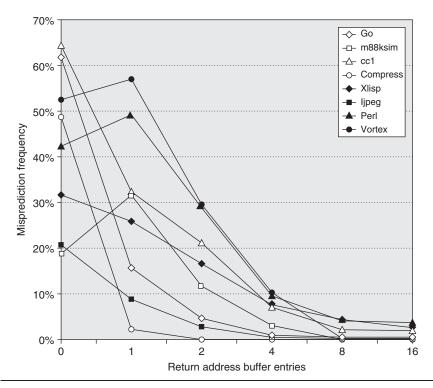
**Figure 3.24** Prediction accuracy for a return address buffer operated as a stack on a number of SPEC CPU95 benchmarks. The accuracy is the fraction of return addresses predicted correctly. A buffer of 0 entries implies that the standard branch prediction is used. Since call depths are typically not large, with some exceptions, a modest buffer works well. These data come from Skadron et al. [1999] and use a fix-up mechanism to prevent corruption of the cached return addresses.
