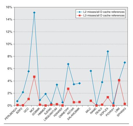
Figure 2.24 The L2 and L3 data cache miss rates for 17 SPECCPU2006 benchmarks are shown relative to all the references to L1, which also includes prefetches, speculative loads that do not complete, and program—generated loads and stores. These data, like the rest in this section, were collected by Professor Lu Peng and Ph.D. student Ying Zhang, both of Louisiana State University.
