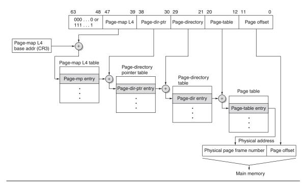
**Figure B.27** The mapping of an Opteron virtual address. The Opteron virtual memory implementation with four page table levels supports an effective physical address size of 40 bits. Each page table has 512 entries, so each level field is 9 bits wide. The AMD64 architecture document allows the virtual address size to grow from the current 48 bits to 64 bits, and the physical address size to grow from the current 40 bits to 52 bits.
