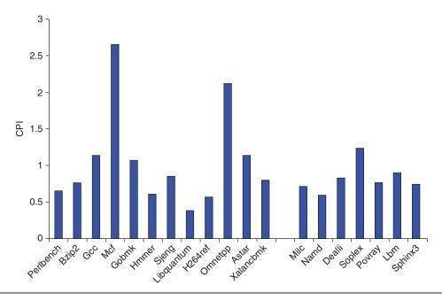
**Figure 3.43** The CPI for the 19 SPECCPU2006 benchmarks shows an average CPI for 0.83 for both the FP and integer benchmarks, although the behavior is quite different. In the integer case, the CPI values range from 0.44 to 2.66 with a standard deviation of 0.77, while the variation in the FP case is from 0.62 to 1.38 with a standard deviation of 0.25. The data in this section were collected by Professor Lu Peng and Ph.D. student Ying Zhang, both of Louisiana State University.
