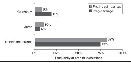
**Figure A.14** Breakdown of control flow instructions into three classes: calls or returns, jumps, and conditional branches. Conditional branches clearly dominate. Each type is counted in one of three bars. The programs and computer used to collect these statistics are the same as those in Figure A.8.
