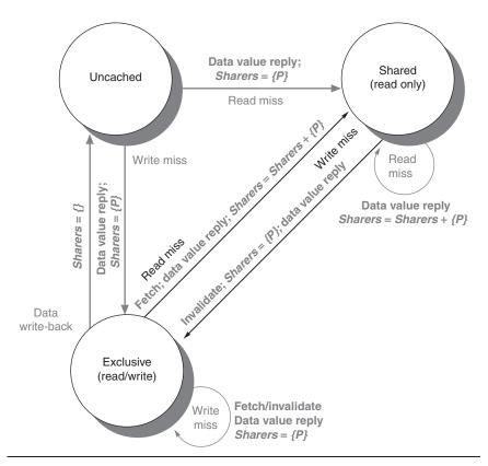
**Figure 5.23** The state transition diagram for the directory has the same states and structure as the transition diagram for an individual cache. All actions are in gray because they are all externally caused. Bold indicates the action taken by the directory in response to the request.
