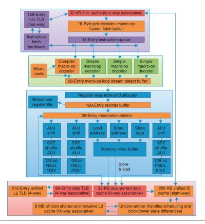
**Figure 3.41** The Intel Core i7 pipeline structure shown with the memory system components. The total pipeline depth is 14 stages, with branch mispredictions costing 17 cycles. There are 48 load and 32 store buffers. The six independent functional units can each begin execution of a ready micro-op in the same cycle.
