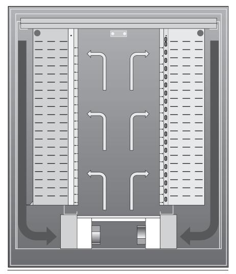
**Figure 6.20** Airflow within the container shown in Figure 6.19. This cross-section diagram shows two racks on each side of the container. Cold air blows into the aisle in the middle of the container and is then sucked into the servers. Warm air returns at the edges of the container. This design isolates cold and warm airflows.
