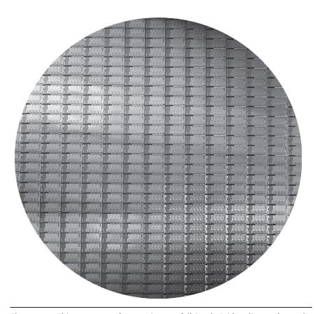
**Figure 1.15** This 300 mm wafer contains 280 full Sandy Bridge dies, each 20.7 by 10.5 mm in a 32 nm process. (Sandy Bridge is Intel's successor to Nehalem used in the Core i7.) At 216 mm<sup>2</sup>, the formula for dies per wafer estimates 282. (Courtesy Intel.)
