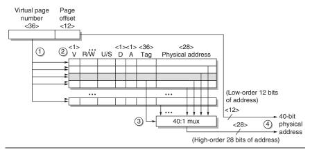
**Figure B.24** Operation of the Opteron data TLB during address translation. The four steps of a TLB hit are shown as circled numbers. This TLB has 40 entries. Section B.5 describes the various protection and access fields of an Opteron page table entry.
