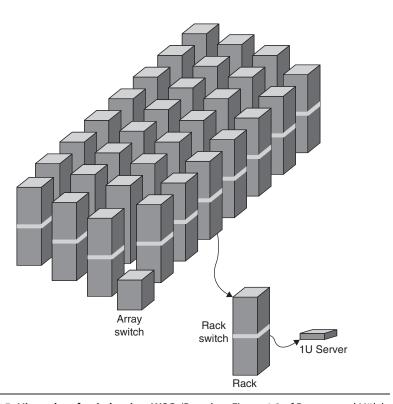
**Figure 6.5** Hierarchy of switches in a WSC. (Based on Figure 1.2 of Barroso and Hölzle [2009].)
