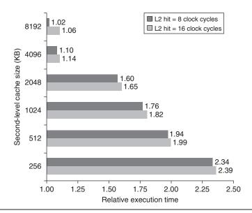
**Figure B.15** Relative execution time by second-level cache size. The two bars are for different clock cycles for an L2 cache hit. The reference execution time of 1.00 is for an 8192 KB second-level cache with a 1-clock-cycle latency on a second-level hit. These data were collected the same way as in Figure B.14, using a simulator to imitate the Alpha 21264.
