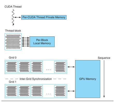
**Figure 4.18 GPU Memory structures.** GPU Memory is shared by all Grids (vectorized loops), Local Memory is shared by all threads of SIMD instructions within a thread block (body of a vectorized loop), and Private Memory is private to a single CUDA Thread.
