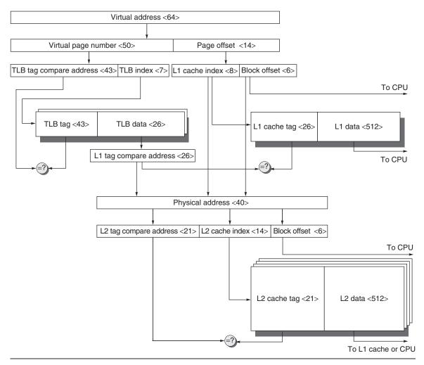
**Figure B.17** The overall picture of a hypothetical memory hierarchy going from virtual address to L2 cache access. The page size is 16 KB. The TLB is two-way set associative with 256 entries. The L1 cache is a direct-mapped 16 KB, and the L2 cache is a four-way set associative with a total of 4 MB. Both use 64-byte blocks. The virtual address is 64 bits and the physical address is 40 bits.
