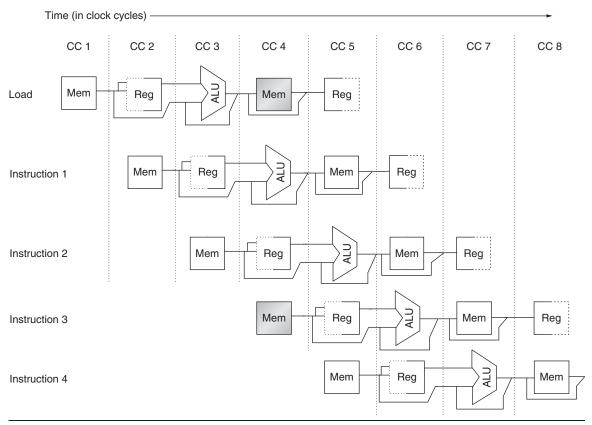
**Figure C.4** A processor with only one memory port will generate a conflict whenever a memory reference occurs. In this example the load instruction uses the memory for a data access at the same time instruction 3 wants to fetch an instruction from memory.
