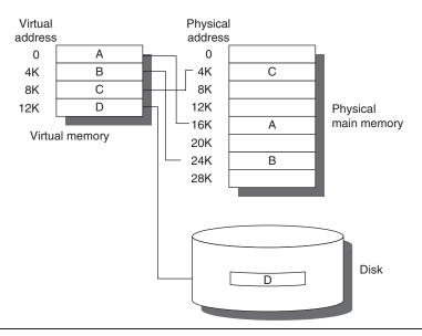
**Figure B.19** The logical program in its contiguous virtual address space is shown on the left. It consists of four pages, A, B, C, and D. The actual location of three of the blocks is in physical main memory and the other is located on the disk.
