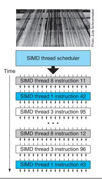
**Figure 4.16 Scheduling of threads of SIMD instructions.** The scheduler selects a ready thread of SIMD instructions and issues an instruction synchronously to all the SIMD Lanes executing the SIMD thread. Because threads of SIMD instructions are independent, the scheduler may select a different SIMD thread each time.
