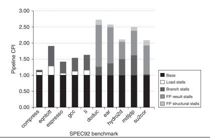
**Figure C.52** The pipeline CPI for 10 of the SPEC92 benchmarks, assuming a perfect cache. The pipeline CPI varies from 1.2 to 2.8. The leftmost five programs are integer programs, and branch delays are the major CPI contributor for these. The rightmost five programs are FP, and FP result stalls are the major contributor for these. Figure C.53 shows the numbers used to construct this plot.
