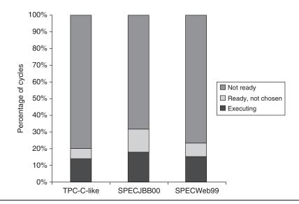
**Figure 3.31** Breakdown of the status on an average thread. "Executing" indicates the thread issues an instruction in that cycle. "Ready but not chosen" means it could issue but another thread has been chosen, and "not ready" indicates that the thread is awaiting the completion of an event (a pipeline delay or cache miss, for example).
