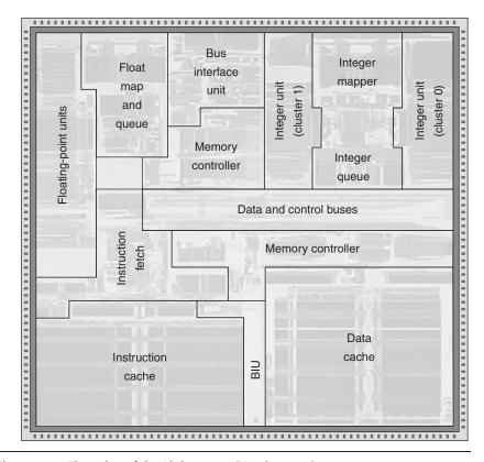
Figure 2.33 Floorplan of the Alpha 21264 [Kessler 1999].
