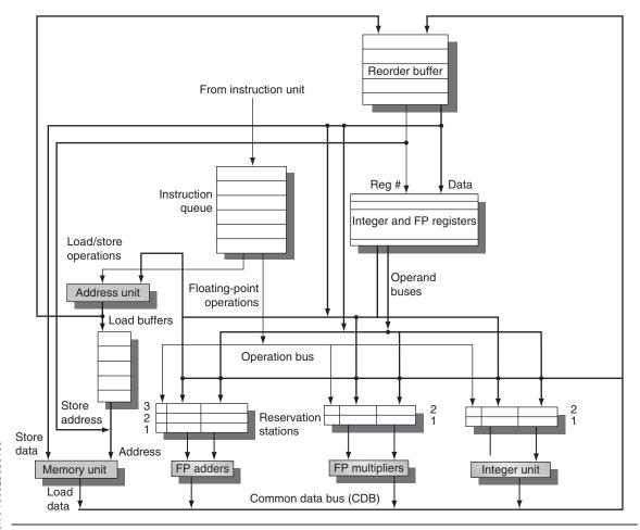
**Figure 3.17** The basic organization of a multiple issue processor with speculation. In this case, the organization could allow a FP multiply, FP add, integer, and load/store to all issues simultaneously (assuming one issue per clock per functional unit). Note that several datapaths must be widened to support multiple issues: the CDB, the operand buses, and, critically, the instruction issue logic, which is not shown in this figure. The last is a difficult problem, as we discuss in the text.
