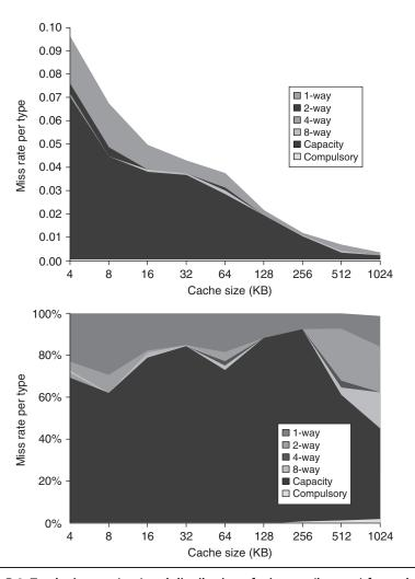
**Figure B.9** Total miss rate (top) and distribution of miss rate (bottom) for each size cache according to the three C's for the data in Figure B.8. The top diagram shows the actual data cache miss rates, while the bottom diagram shows the percentage in each category. (Space allows the graphs to show one extra cache size than can fit in Figure B.8.)
