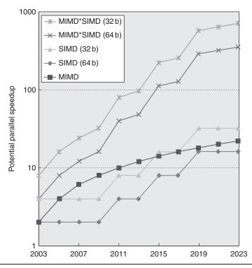
**Figure 4.1** Potential speedup via parallelism from MIMD, SIMD, and both MIMD and SIMD over time for x86 computers. This figure assumes that two cores per chip for MIMD will be added every two years and the number of operations for SIMD will double every four years.
