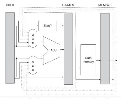
**Figure C.27** Forwarding of results to the ALU requires the addition of three extra inputs on each ALU multiplexer and the addition of three paths to the new inputs. The paths correspond to a bypass of: (1) the ALU output at the end of the EX, (2) the ALU output at the end of the MEM stage, and (3) the memory output at the end of the MEM stage.
