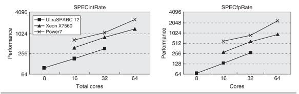
**Figure 5.28** The performance on the SPECRate benchmarks for three multicore processors as the number of processor chips is increased. Notice for this highly parallel benchmark, nearly linear speedup is achieved. Both plots are on a log-log scale, so linear speedup is a straight line.
