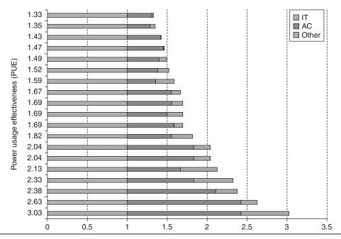
**Figure 6.11** Power utilization efficiency of 19 datacenters in 2006 [Greenberg et al. 2006]. The power for air conditioning (AC) and other uses (such as power distribution) is normalized to the power for the IT equipment in calculating the PUE. Thus, power for IT equipment must be 1.0 and AC varies from about 0.30 to 1.40 times the power of the IT equipment. Power for "other" varies from about 0.05 to 0.60 of the IT equipment.
