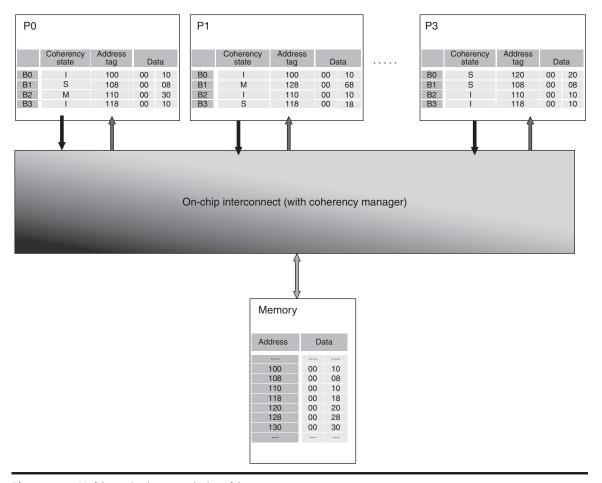
Figure 5.35 Multicore (point-to-point) multiprocessor.
