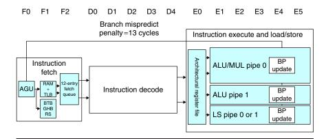
**Figure 3.36** The basic structure of the A8 pipeline is 13 stages. Three cycles are used for instruction fetch and four for instruction decode, in addition to a five-cycle integer pipeline. This yields a 13-cycle branch misprediction penalty. The instruction fetch unit tries to keep the 12-entry instruction queue filled.
