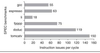
**Figure 3.26** ILP available in a perfect processor for six of the SPEC92 benchmarks. The first three programs are integer programs, and the last three are floating-point programs. The floating-point programs are loop intensive and have large amounts of loop-level parallelism.
