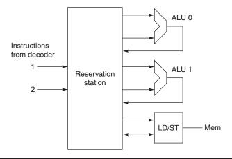
Figure 3.55 An out-of-order microarchitecure.
