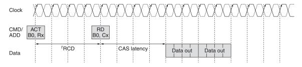
Figure 2.31 DDR2 SDRAM timing diagram.
