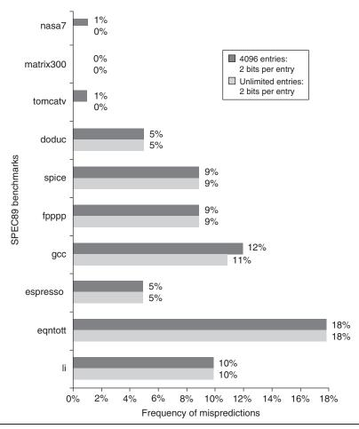
**Figure C.20** Prediction accuracy of a 4096-entry 2-bit prediction buffer versus an infinite buffer for the SPEC89 benchmarks. Although these data are for an older version of a subset of the SPEC benchmarks, the results would be comparable for newer versions with perhaps as many as 8K entries needed to match an infinite 2-bit predictor.
