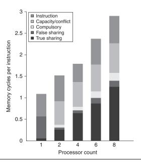
**Figure 5.14** The contribution to memory access cycles increases as processor count increases primarily due to increased true sharing. The compulsory misses slightly increase since each processor must now handle more compulsory misses.
