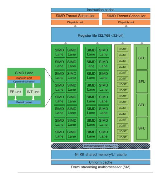
**Figure 4.20** Block diagram of the multithreaded SIMD Processor of a Fermi GPU. Each SIMD Lane has a pipelined floating-point unit, a pipelined integer unit, some logic for dispatching instructions and operands to these units, and a queue for holding results. The four Special Function units (SFUs) calculate functions such as square roots, reciprocals, sines, and cosines.
