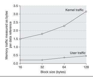
**Figure 5.19** The number of bytes needed per data reference grows as block size is increased for both the kernel and user components. It is interesting to compare this chart against the data on scientific programs shown in Appendix I.
