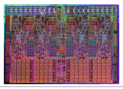
**Figure 1.13** Photograph of an Intel Core i7 microprocessor die, which is evaluated in Chapters 2 through 5. The dimensions are 18.9 mm by 13.6 mm (257 mm<sup>2</sup>) in a 45 nm process. (Courtesy Intel.)
