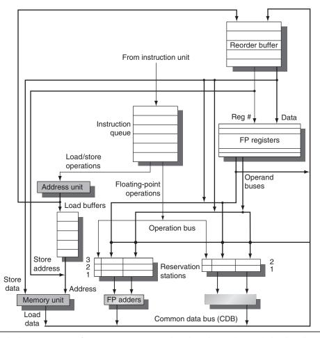
**Figure 3.11** The basic structure of a FP unit using Tomasulo's algorithm and extended to handle speculation. Comparing this to Figure 3.6 on page 173, which implemented Tomasulo's algorithm, the major change is the addition of the ROB and the elimination of the store buffer, whose function is integrated into the ROB. This mechanism can be extended to multiple issue by making the CDB wider to allow for multiple completions per clock.
