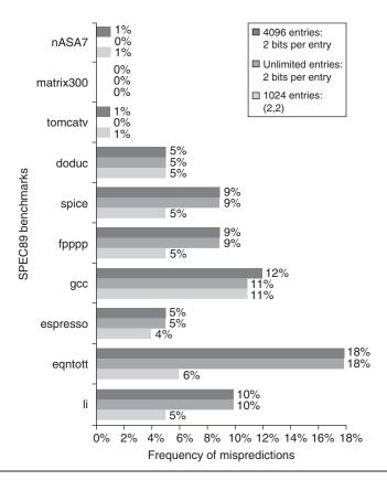
**Figure 3.3** Comparison of 2-bit predictors. A noncorrelating predictor for 4096 bits is first, followed by a noncorrelating 2-bit predictor with unlimited entries and a 2-bit predictor with 2 bits of global history and a total of 1024 entries. Although these data are for an older version of SPEC, data for more recent SPEC benchmarks would show similar differences in accuracy.
