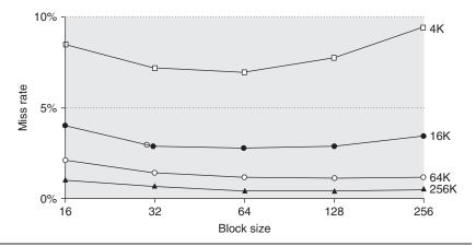
**Figure B.10** Miss rate versus block size for five different-sized caches. Note that miss rate actually goes up if the block size is too large relative to the cache size. Each line represents a cache of different size. Figure B.11 shows the data used to plot these lines. Unfortunately, SPEC2000 traces would take too long if block size were included, so these data are based on SPEC92 on a DECstation 5000 [Gee et al. 1993].
