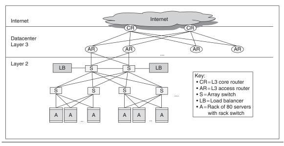
**Figure 6.8** The Layer 3 network used to link arrays together and to the Internet [Greenberg et al. 2009]. Some WSCs use a separate *border router* to connect the Internet to the datacenter Layer 3 switches.
