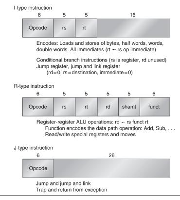
**Figure A.22 Instruction layout for MIPS.** All instructions are encoded in one of three types, with common fields in the same location in each format.
