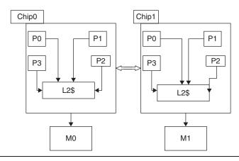
Figure 5.37 Multichip, multicore multiprocessor with DSM.
