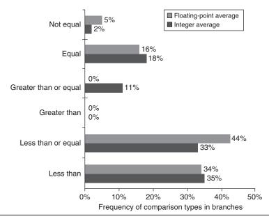
**Figure A.17** Frequency of different types of compares in conditional branches. Less than (or equal) branches dominate this combination of compiler and architecture. These measurements include both the integer and floating-point compares in branches. The programs and computer used to collect these statistics are the same as those in Figure A.8.
