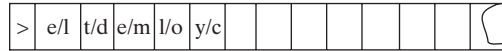
Figure 1.5. To simulate a machine M with alphabet \Gamma that has tapes infinite in both directions, we use a machine \tilde{M} with alphabet \Gamma^2 whose tapes encode the “folded” version of M 's tapes.
