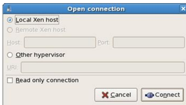
Figure 7.9. The Open Connection dialog allows you to connect to local or remote Xen hosts.
