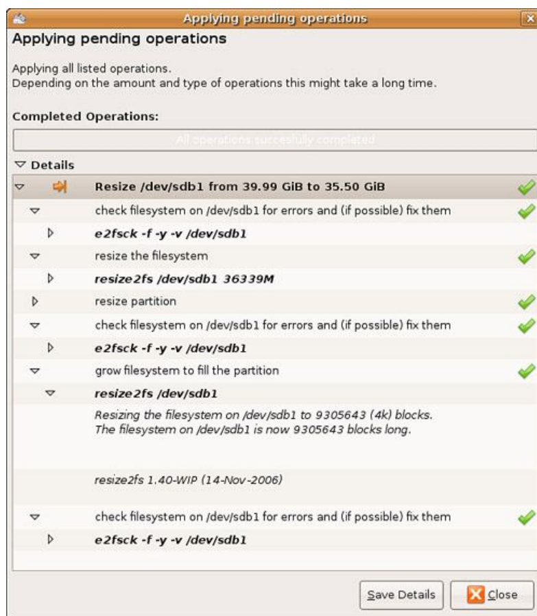
Figure 5.7. Clicking Apply brings up the Pending Operation dialog. We have expanded out some of the details you can see the operation and commands that go into doing the actual resize operation.
