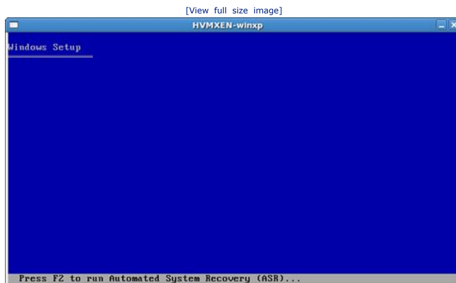
Figure 7.1. The Windows XP setup screen loads within the VNC console of our HVM DomU guest.
