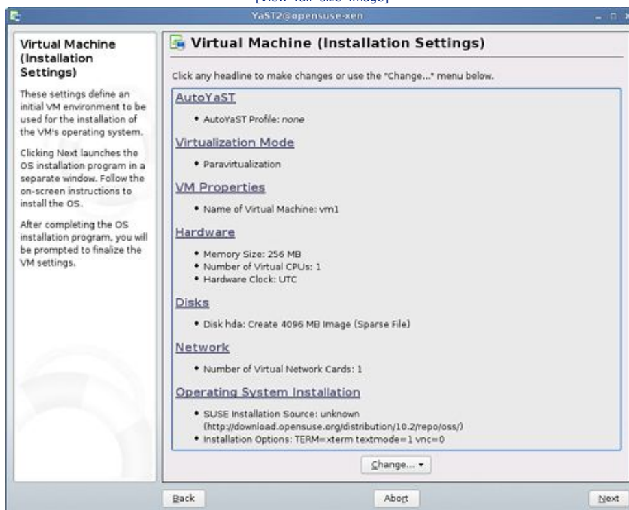
Figure 7.8. The Virtual Machine (Installation Settings) window lets you install an operating system just as you would normally install OPEN SUSE.
