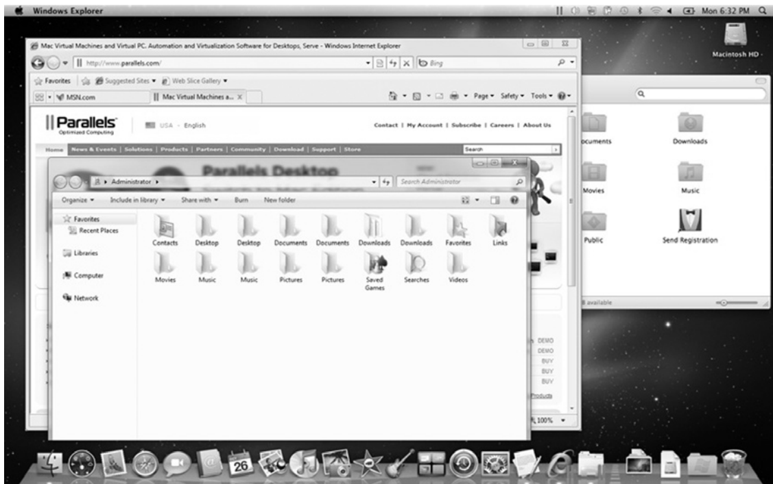
Figure 3.7 Parallels for Mac Running a Windows Vista Virtual Environment
