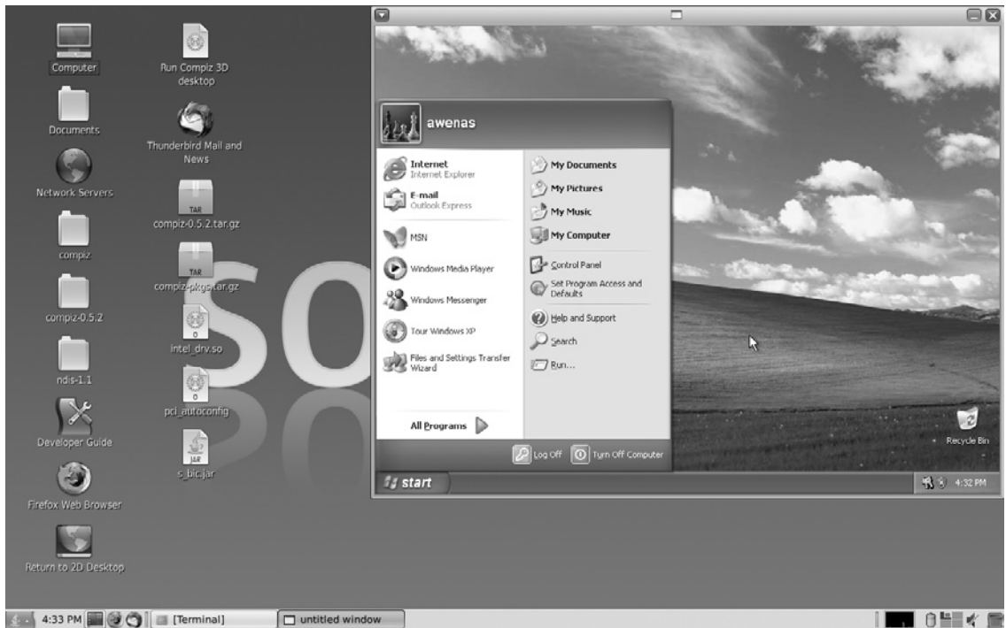
Figure 3.10 Xen VMM Running a Windows XP Virtual Environment inside Linux
