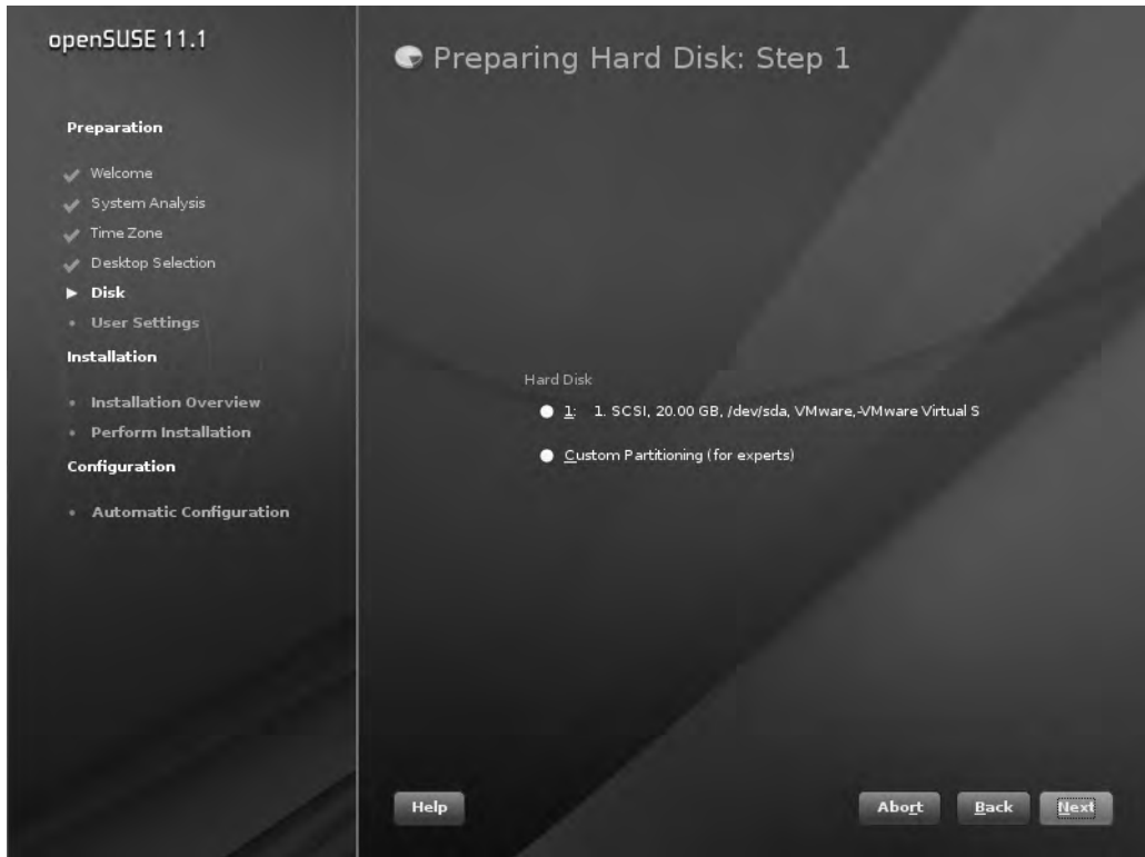
Figure A-2. Select Custom Partitioning (for experts) to create your own disk layout.
