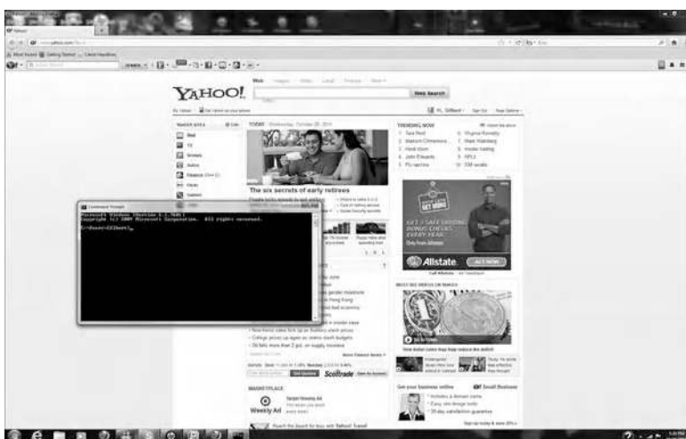
Figure 5.3 The Command Prompt window can be placed in the forefront by clicking on its icon on the taskbar.
