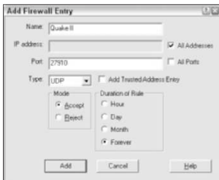
Figure 15-17: Quake II port rule.
