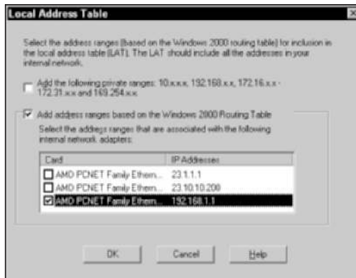
Figure 16-4: The Local Address Table construction dialog box.
