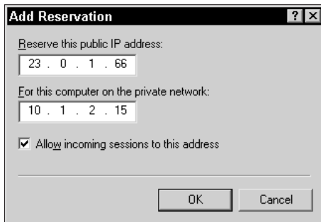
Figure 13-4: Windows 2000 NAT static address mapping.
