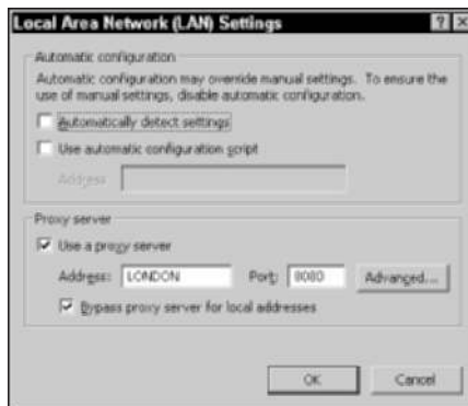
Figure 16-8: The LAN Settings dialog box in Internet Explorer.
