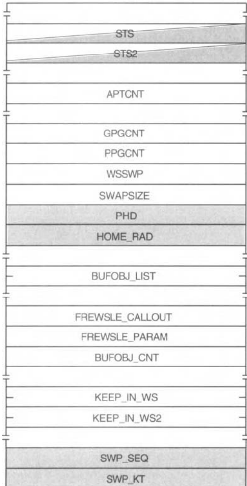
Figure 2.1 PCB and KTB (Shaded) Fields Related to Memory Management
