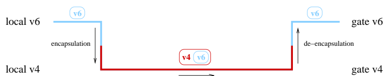
Figure 11-7. A frequently used method for transition is tunneling IPv6 in IPv4 packets
