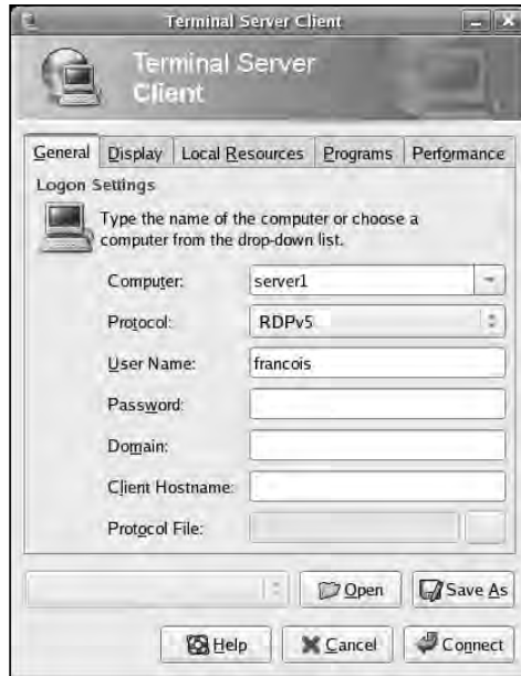
Figure 13-2: Terminal Server Client (tsclient) connects to Windows desktops
