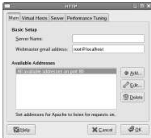
Figure 2-2: In Fedora Core, configure the Apache HTTP server from this dialog box.
