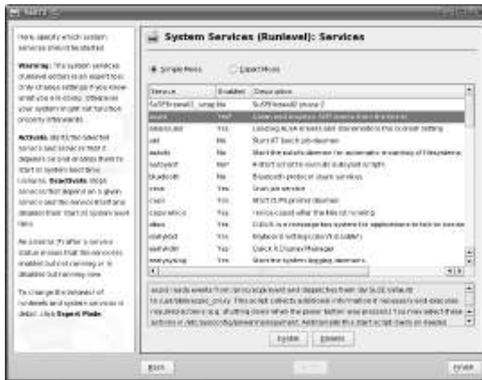
Figure 1-3: In SUSE, use this YaST window to specify services that start at boot time.
