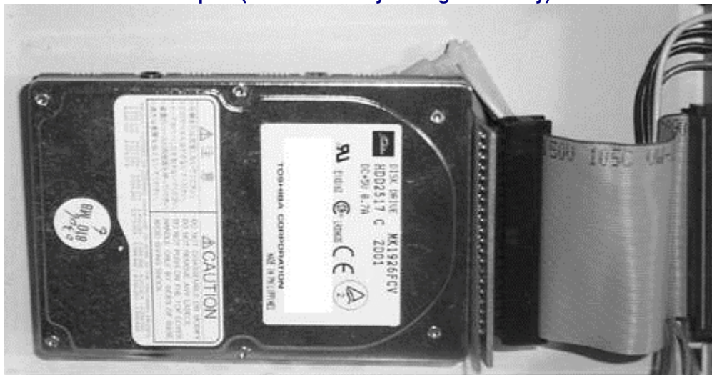
Figure 2.11. A 44-pin ATA laptop drive connected to a 40-pin ATA ribbon cable using an adaptor (Photo courtesy of Eoghan Casey).
