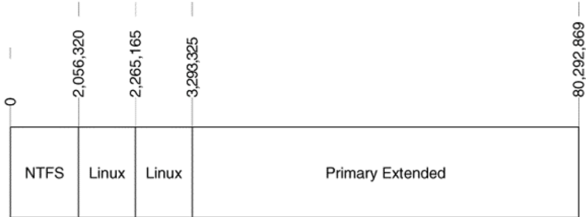
Figure 5.5. Disk layout after processing the first partition table in example (not to scale).
