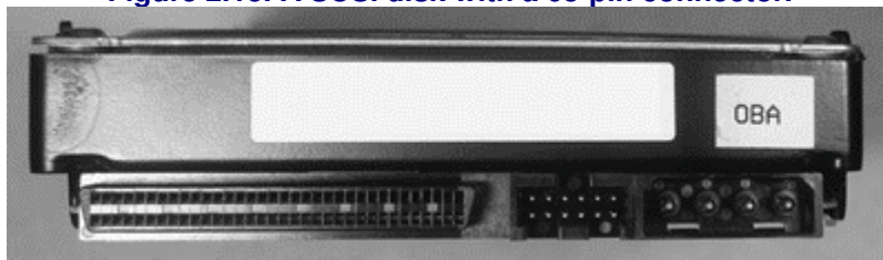
Figure 2.15. A SCSI disk with a 68-pin connector.
