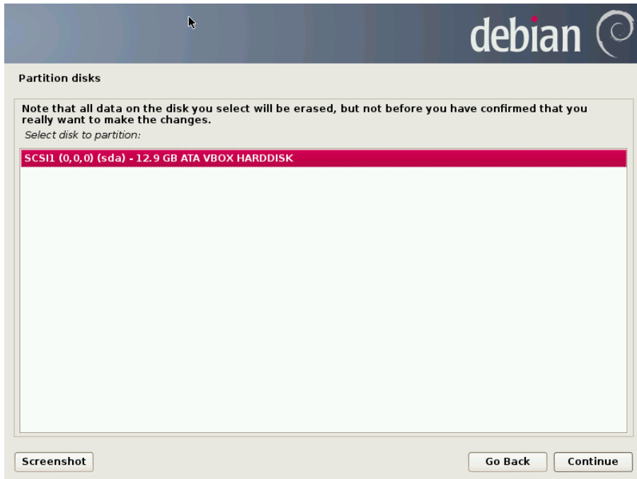
Figure 4.8 Disk to use for guided partitioning
