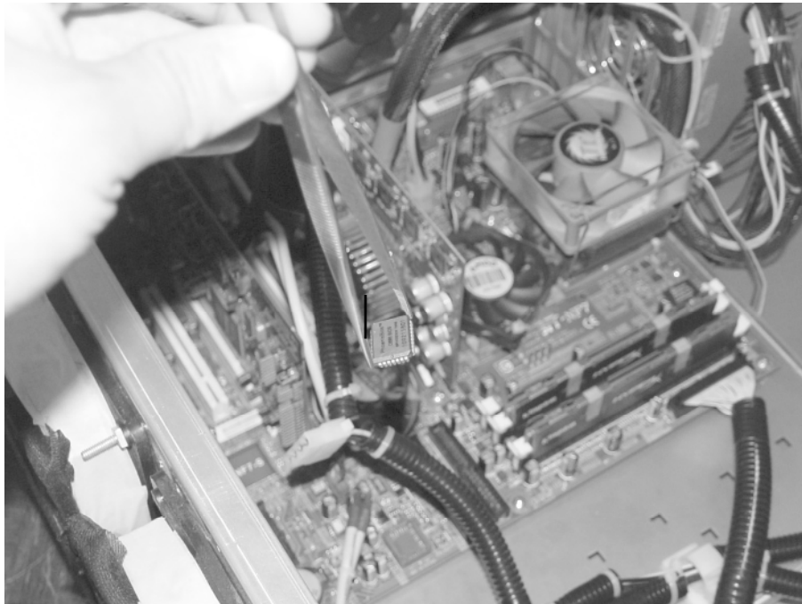
Inserting the corrupted BIOS chip. (Photo by author)
