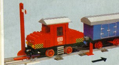
Automatic shunting. A trip post flicks the switch from forward to reverse.
