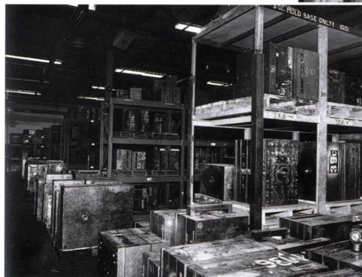
Hundreds of classic Revell-Monogram mold ('mold') tools in store at Morten Grove.
