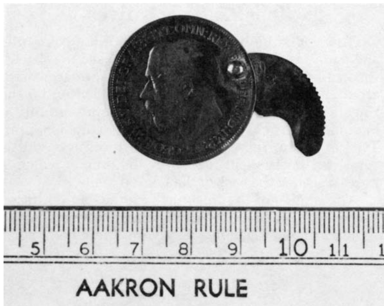
Coin knife with alternate mounting of the cutter on the tail side. (Photo courtesy of Keith Melton.)
