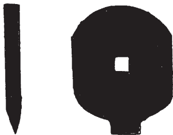
Combination file and screwdriver. This is the prototype constructed from a machinist's file. The center hole can be used as a drill brace. (CIA illustration.)
