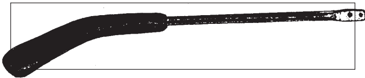
Scroll saw blade concealed in the steel tube of an eyeglass temple piece. (CIA illustration.)
