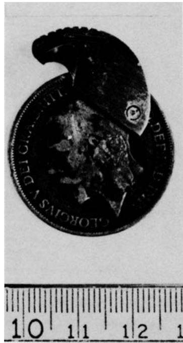
Coin knife with gullet blade and pivot pin mounted on the head side. (Photo courtesy of Keith Melton.)
