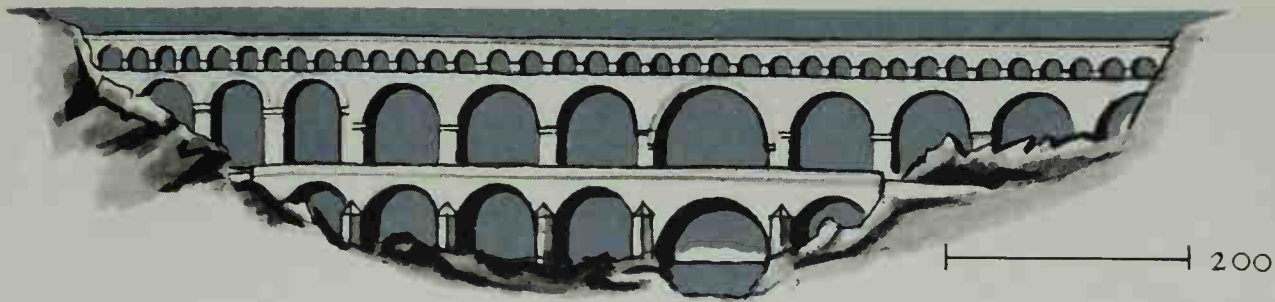
Arches supported on piers: Aqueduct, Pont du Gard, Nîmes, c.A.D. 150
