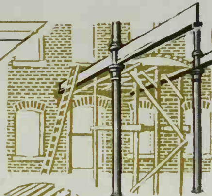
Cotton mill, Manchester, 1801. Cast-iron columns & beams James Watt (1736-1819) & Matthew Boulton (1728-1809)
