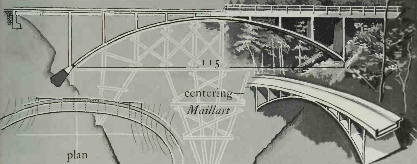
Schwandbach stiffened arch Bridge, Berne, Switzerland, 1933 Maillart
