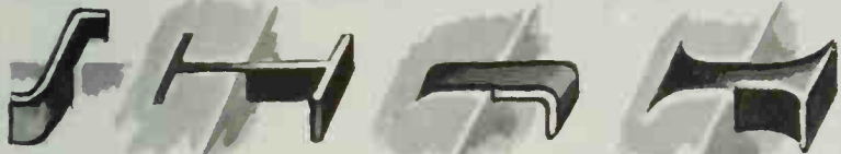
METAL CRAMPS set in molten lead
