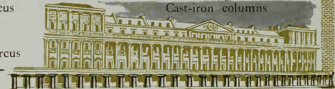
B Carlton House Terrace, 1827 Cast-iron Doric columns
