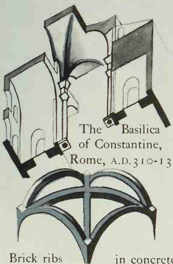
Construction of arches on piers with non-constructural facing of columns and entablature
