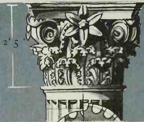
The Temple of Vesta, Tivoli (restored), 27 B.C.-A.D. 14 Foundations: tufa. Podium and walls: concrete. Columns and door: travertine. Roof: probably a low concrete dome
