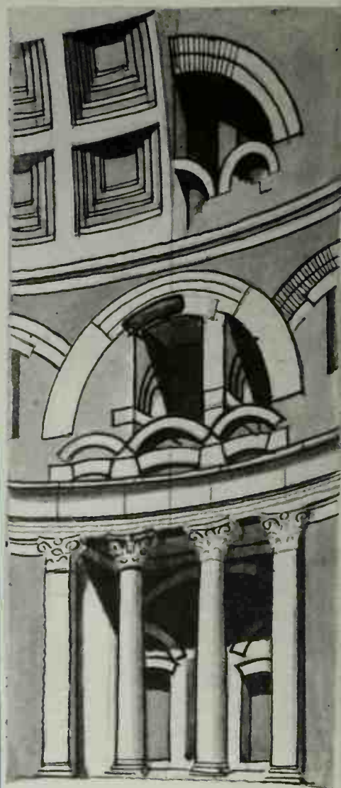
Concealed brick arches link together 8 massive brick piers supporting the dome
