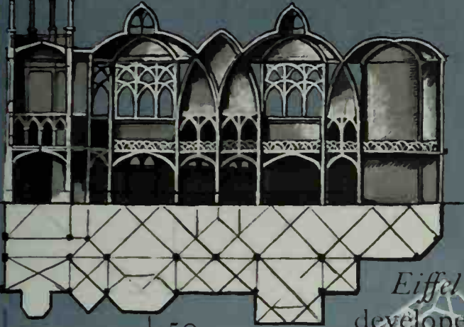
S. Jean de Montmartre, Paris, 1894: first church in reinforced concrete Anatole de Baudot (1834-1915)
