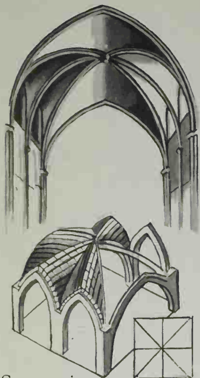
Sixpartite or six-part ribbed vault Canterbury Cathedral choir, 1275-1278
