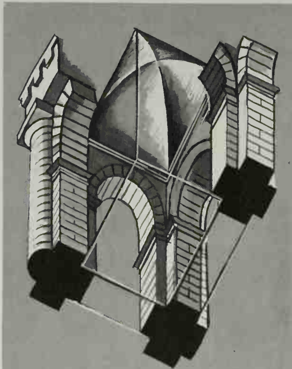
Cloister vault of concrete supported on cruciform piers Tabularium, Rome, 78 B.C.
