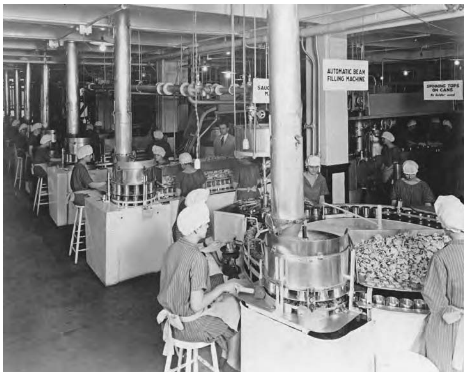
Automated filling in the baked bean department, 1911 (courtesy Benson Ford Research Center, The Henry Ford, 53.41 Box 12).
