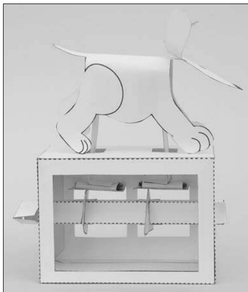
Figure 10-22: The pushrods attach to the cam followers.
