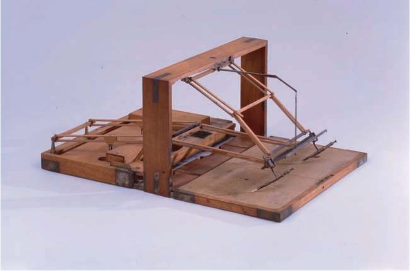
Figure 2.12. Thomas Jefferson Polygraph (i.e., pantograph), 1804. Slanted pen holders are visible, as are parallelograms.
