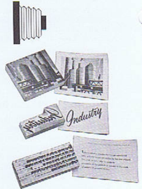
3 The engraver makes a square halftone plate of the tonal illustration and a line plate for the heading, and a proof of each is pulled. The typesetter sets type for the body text and pulls a galley proof.
