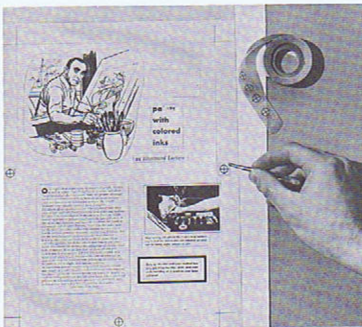
21 Stick register marks on both sides and the bottom of the mechanical. Then, for color separation, tape a clear acetate overlay on the mechanical and position register marks on this exactly over the ones beneath. Register marks can be drawn with a ruling pen, T-square and triangle, but pre-printed ones are real timesavers.
