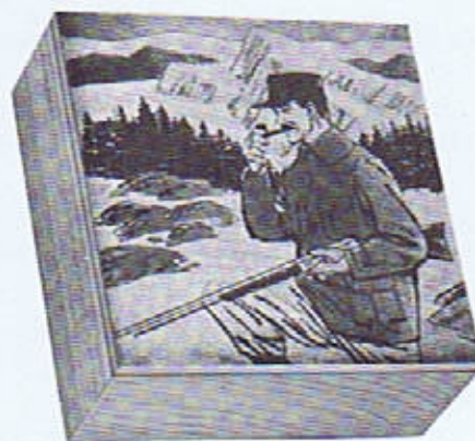
This is a halftone engraving made from a tonal drawing of the same subject as above. It has been blocked type high and is ready for printing by letterpress.
