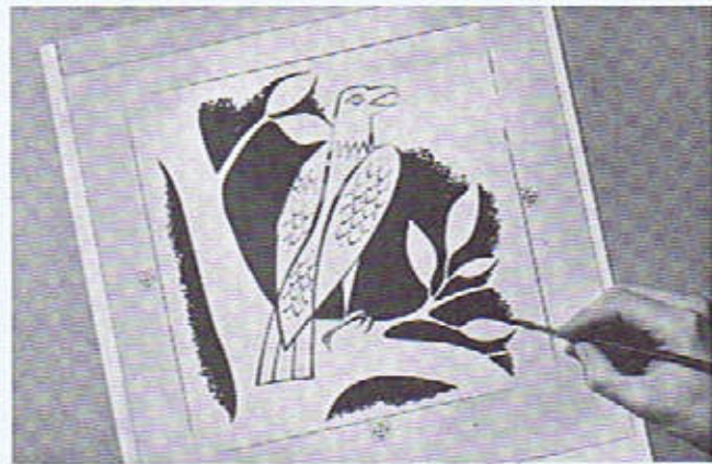
2 Tape an acetate overlay over the mechanical and add register marks. This is the overlay for color and is pointed with black ink. Where this comes up to the art on the mechanical beneath, let the black on the acetate overlap the lines of the photostat a little to assure perfect register. Add a tissue overlay and indicate color separation. (Use a "treated" acetate for inking, and keep it free of fingerprints or ink will skip.)
