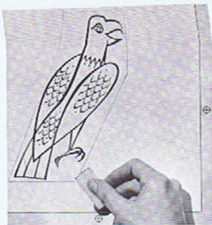
1 Rule holding lines and cement a stat of the black art in position on the mechanical. Then position register marks.
