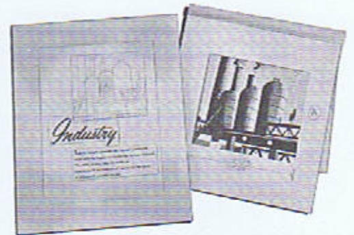
3 A mechanical is made. A photostat or lucy drawing of the tonal illustration, a photostat of the headline, and the repro proof of the body text are pasted in the position they will occupy in the printed piece.
