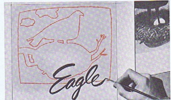
2 Now draw or cement your line art in position on the mechanical. Use opaque white to paint a break between the red key lines and your black line art. Use a tissue overlay for instructions to the platemaker.
