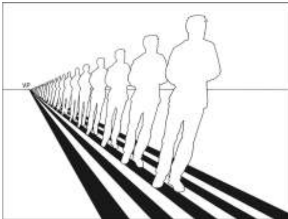
Figure 11-8: Subjects become smaller until they seem to disappear at the vanishing point.
