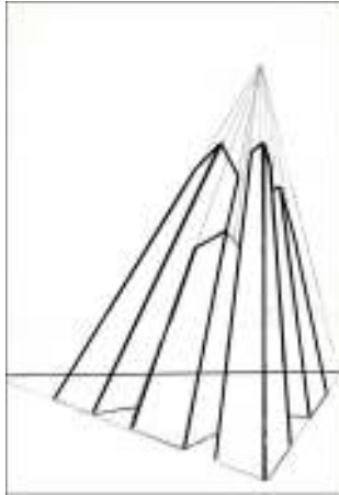
Figure 11-22: Using perspective lines to draw the other buildings that will line the street.
