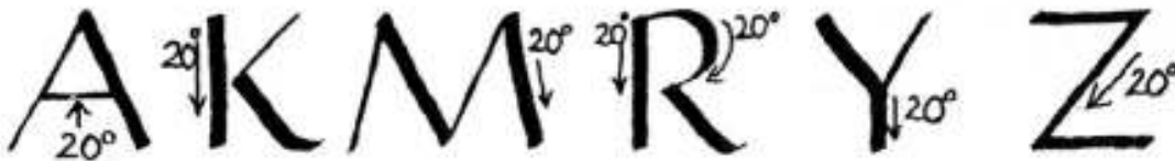
Figure 9-10: Select parts of a, k, m, r, y, and z use the 20- degree angle as indicated.
