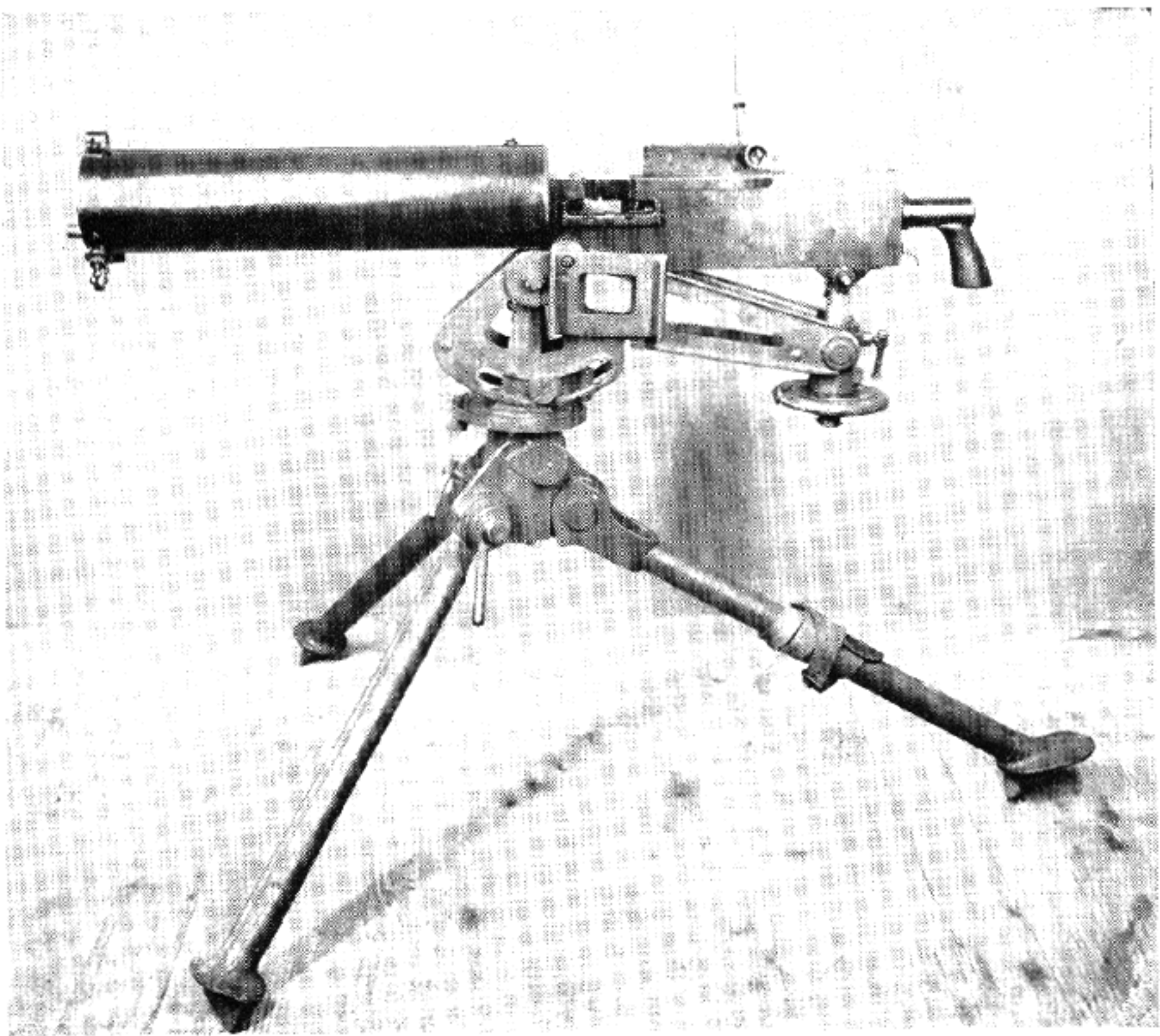
The Browning .30 caliber water cooled machine gun.
