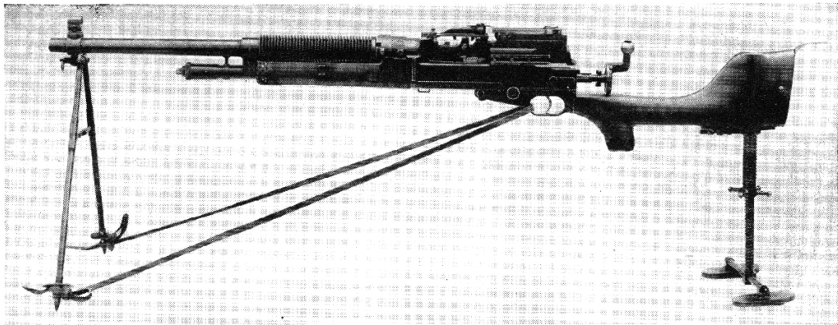
The Automatic Machine Rifle, Caliber .30, Model of 1909, which was the standard light machine gun of our Army at the beginning of World War I. This light Hotchkiss gun, known also as the Benet-Mercié, from the names of two Hotchkiss Company engineers who developed it, was superseded by the Browning Automatic Rifle.
