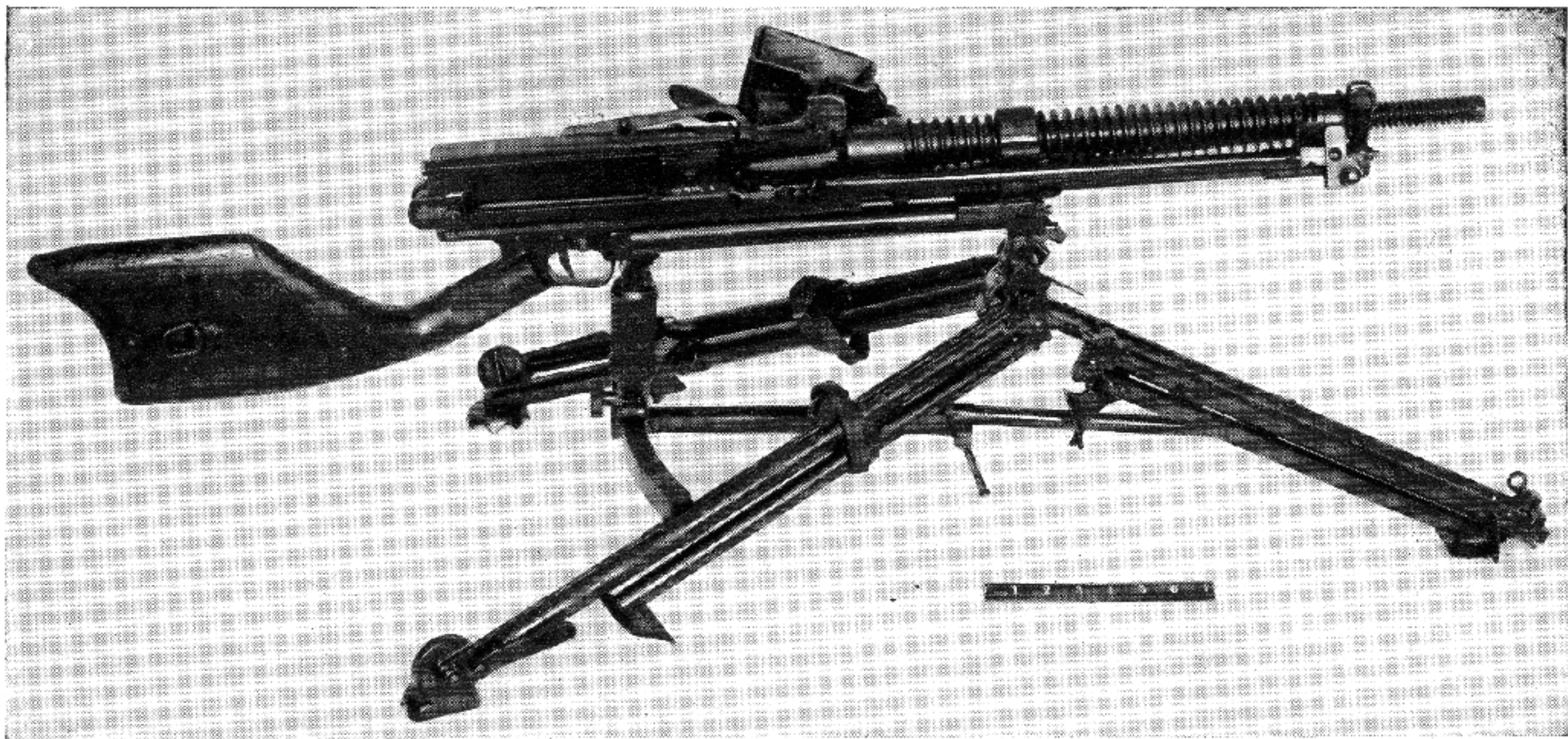
Japanese Nambu machine gun, Model 11 (1922). Except for the hopper feed, it follows the Hotchkiss principle of design.
