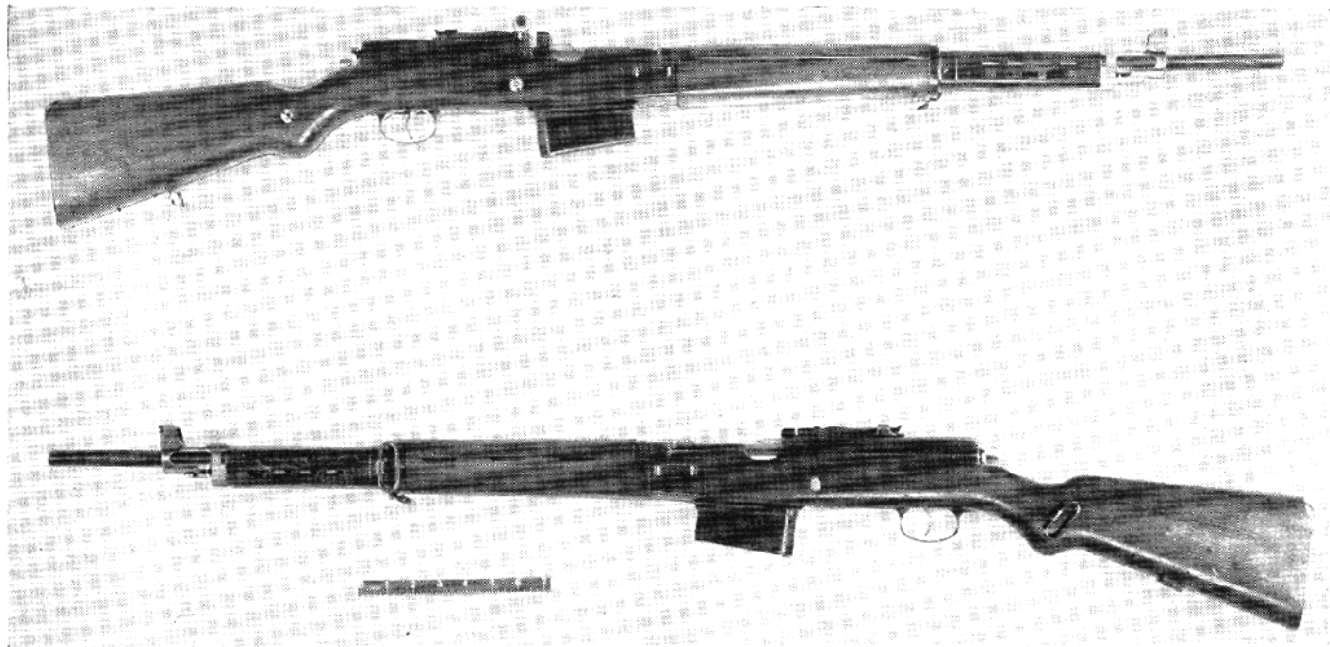
A second type of Czech experimental semiautomatic rifle found in Germany during World War II. It is made in the regular German 7.92 caliber, and is gas operated.
