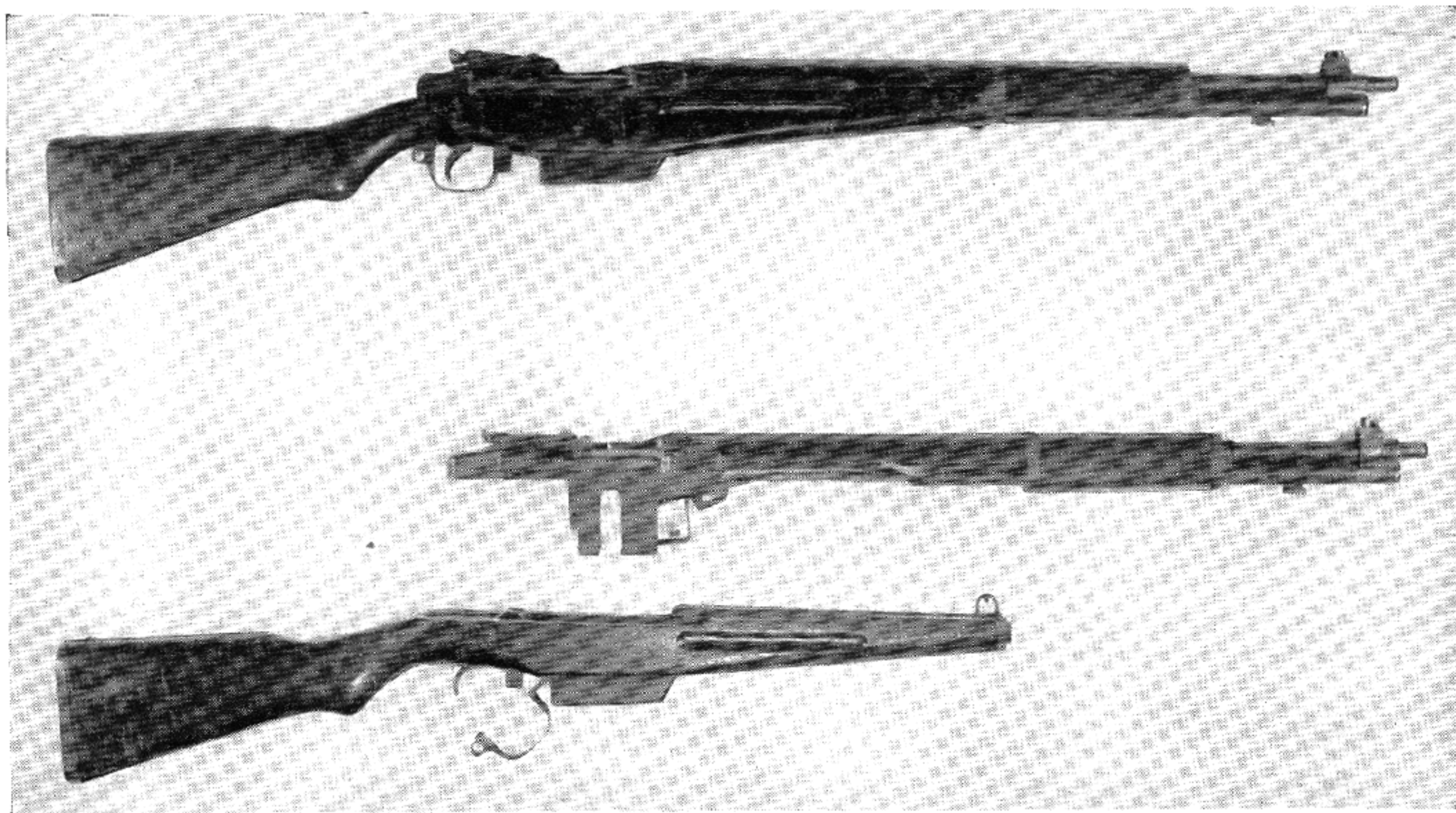
Japanese copy of the U. S. Garand M1 rifle. Guns like this, differing from the U. S. M1 only in minor details were found in the Japanese service towards the close of the war. Main differences were the caliber, which was the standard Japanese 7.7mm; the rear sight, which was of the ramp type, and the magazine, which was arranged for loading by having the cartridges stripped out of a clip as is done in the M1903 Springfield.
