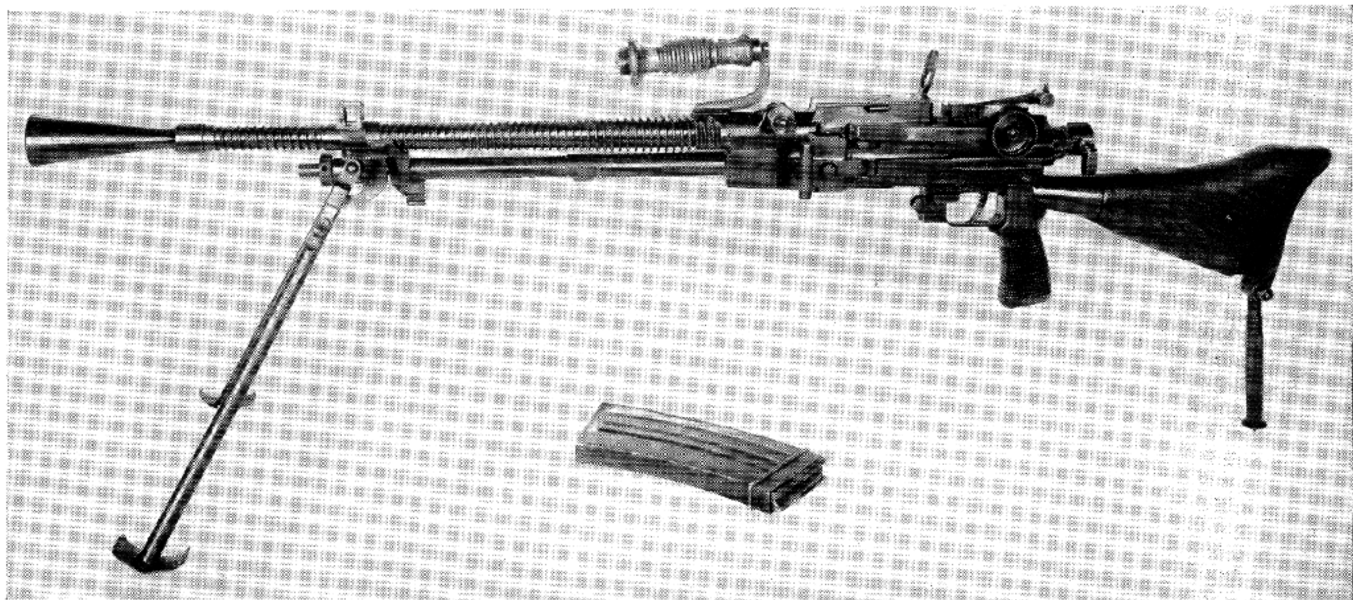
Japanese Model 99 (1939) light machine gun. This was the latest Japanese light machine gun to be used in World War II. It is gas operated, weighs about 20 pounds, and is simple and effective in design.
