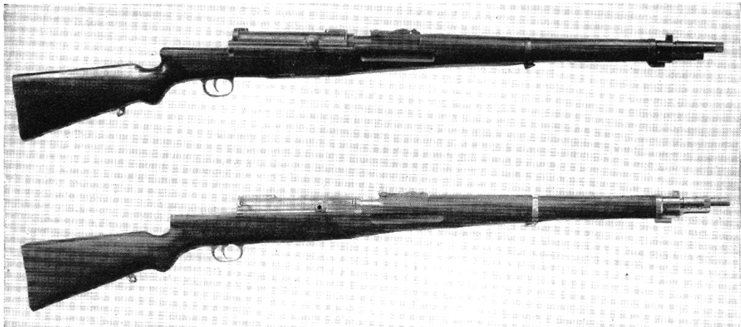
Two models of the Liu semiautomatic rifle tested at Springfield in 1918. This Chinese designed rifle submitted by General Liu follows the Bang principles very closely.
