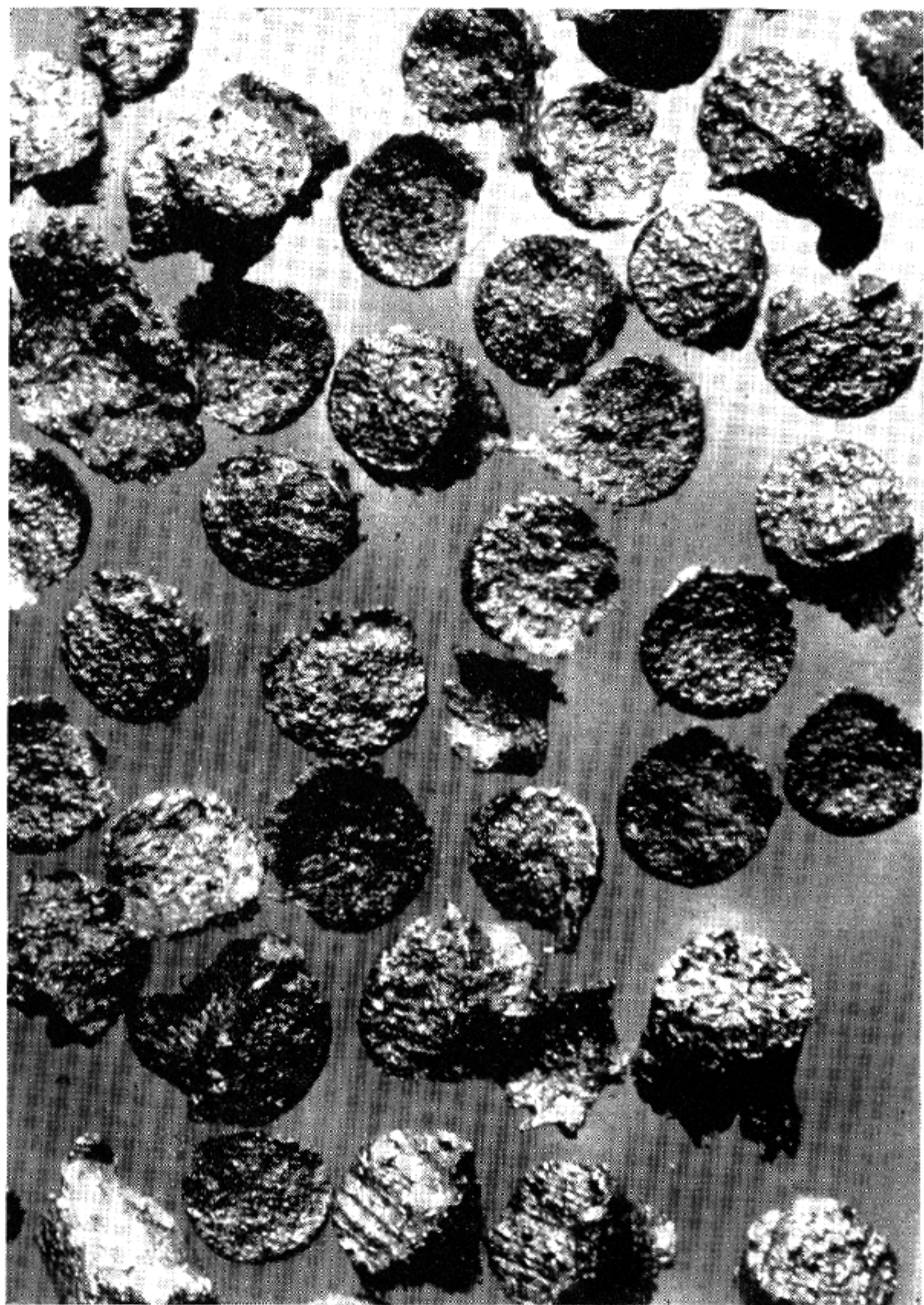
A popular dense pistol powder, DuPont's Pistol Powder No. 5. It consists of fine flakes of nitrocellulose. Magnified 20 times.
