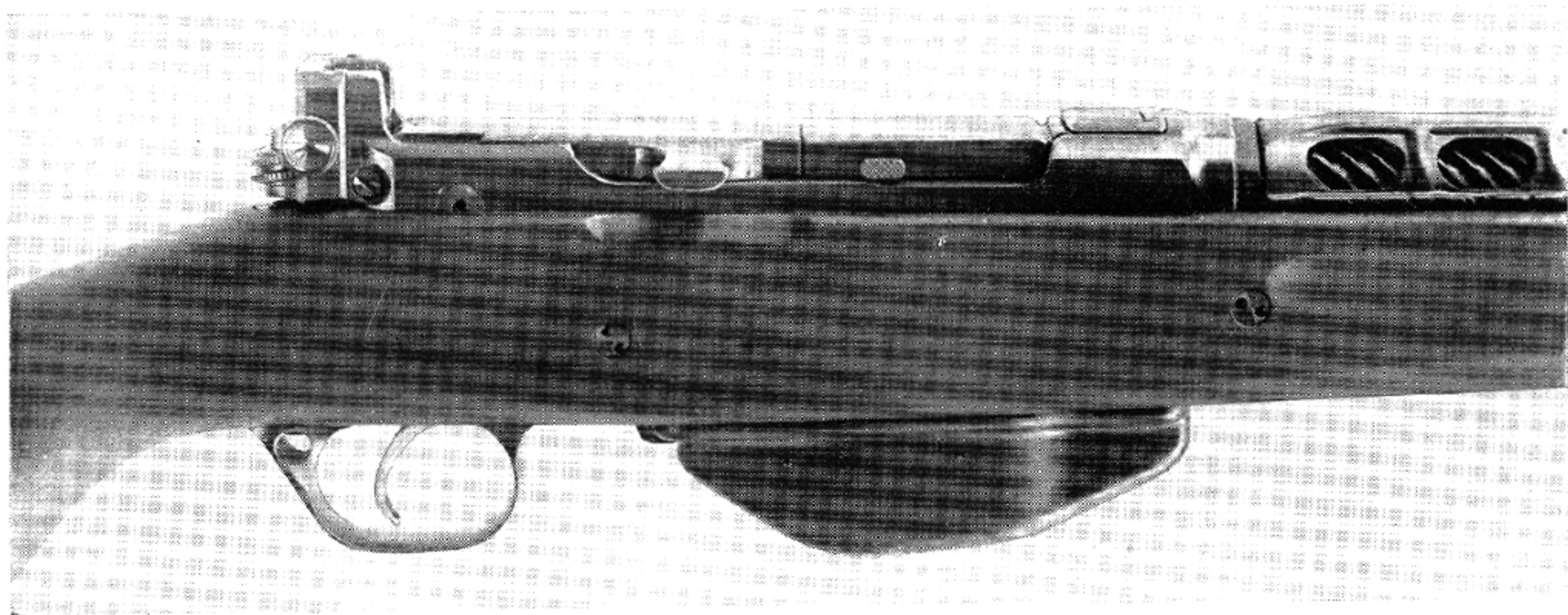
Pedersen .276 semiautomatic, showing action in closed position.
