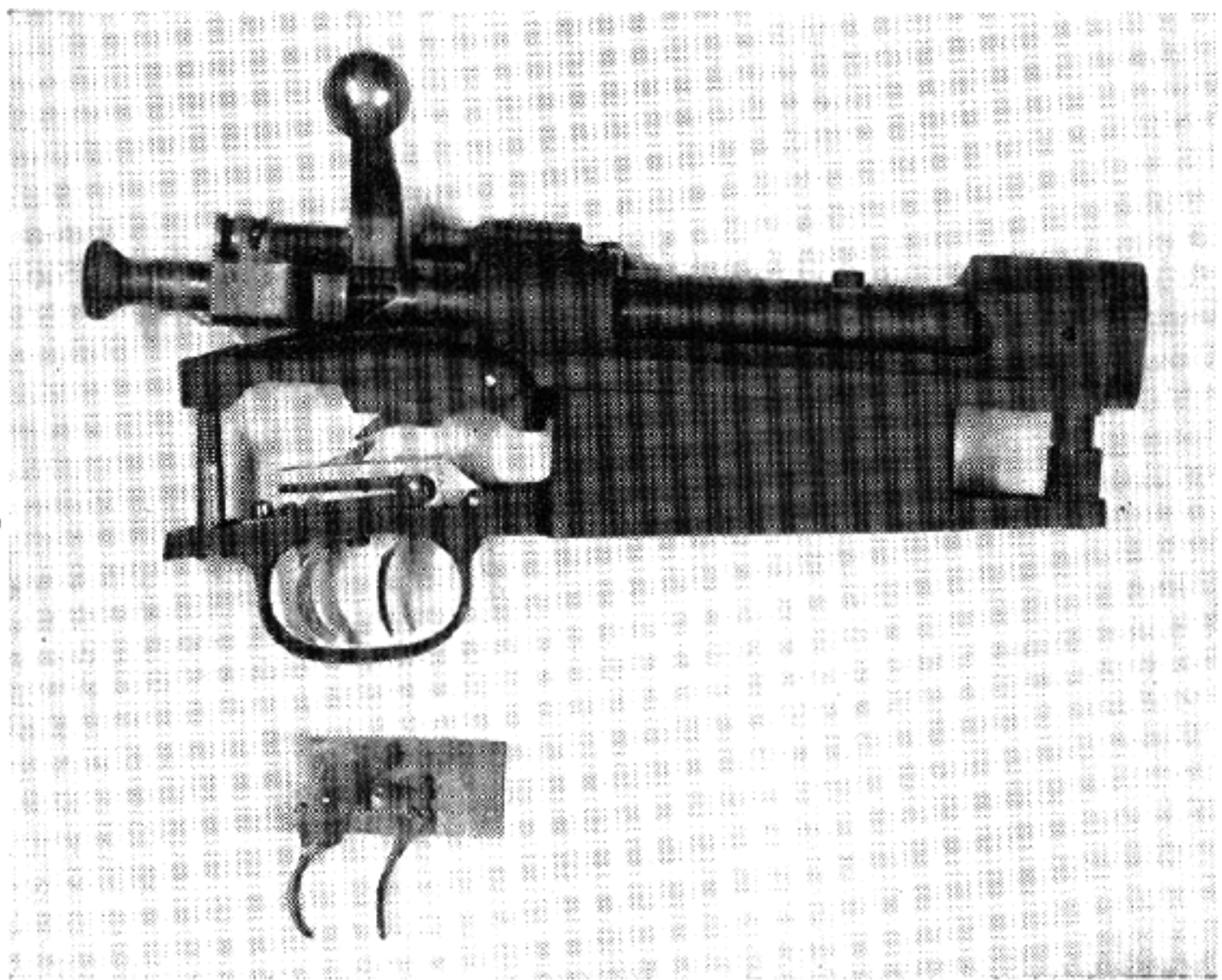
Figure 3. Woody trigger assembled in rifle action.
