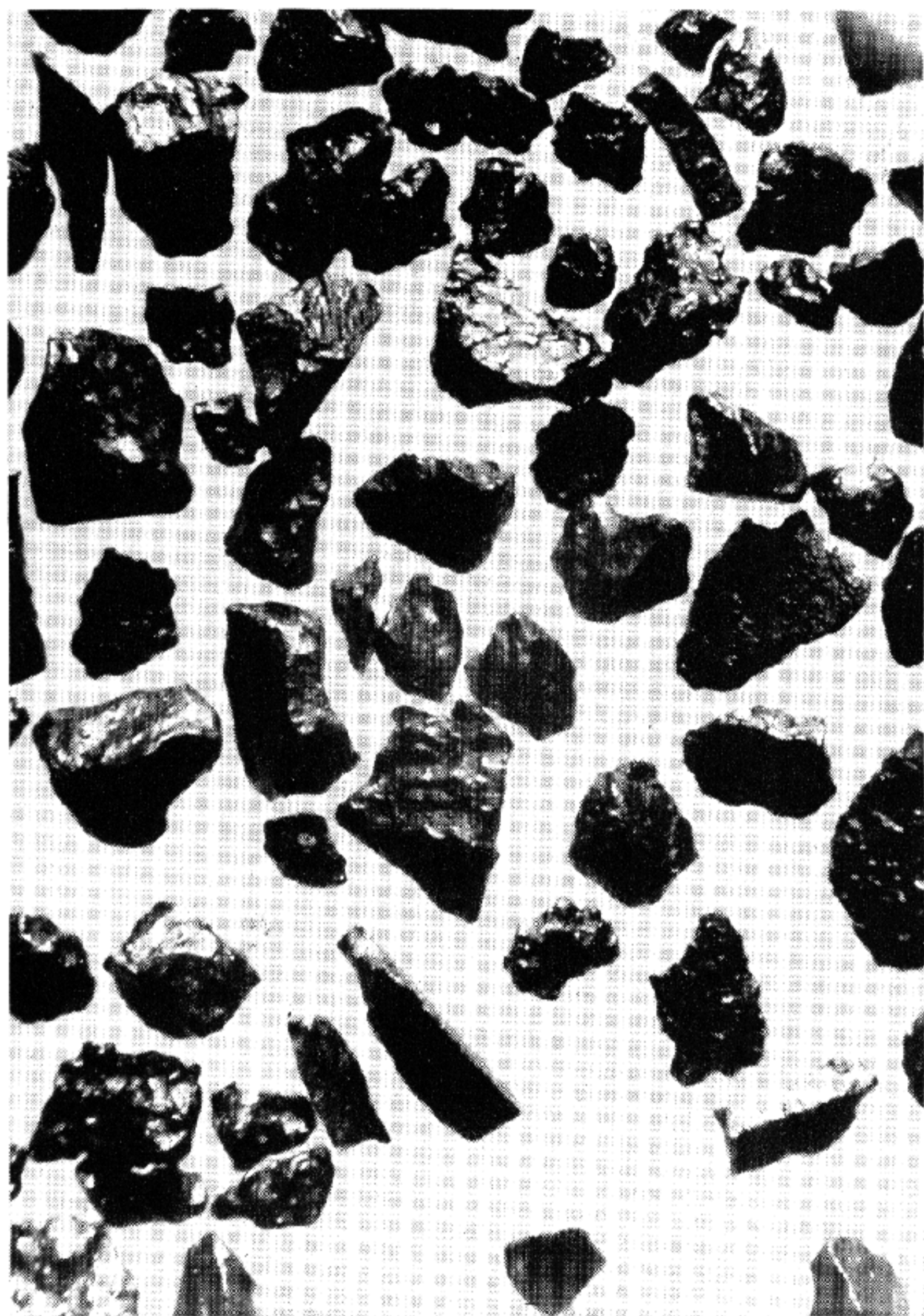
Black powder of medium granulation, suitable for large caliber pistol cartridges. Black powder, grain size FFG. Magnified 20 times.
