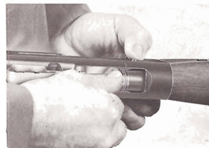
1 Loosen take-down screw by turning it in counter-clockwise direction.
