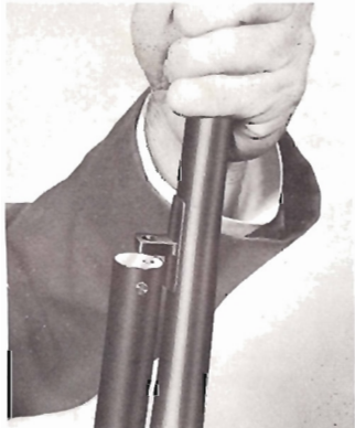
3 Apply firm downward pressure and twist barrel one quarter turn until threaded holes in magazine tube and barrel lug line up.
