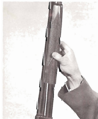
2 Slip the forearm off of magazine tube.
