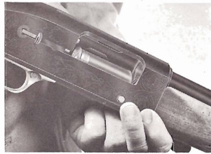
3 Drop a shot shell into loading port.
