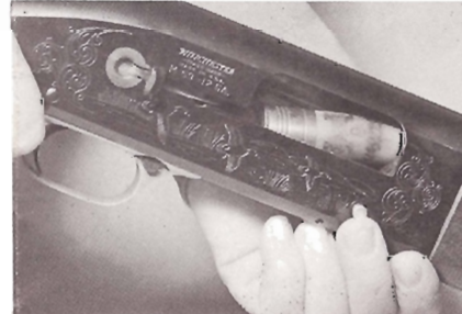
4 Replace forearm on magazine tube and seat against receiver. Take-down screw will enter hole in barrel lug.
