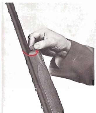
1 Loosen take-down screw by turning it in counter-clockwise direction.
