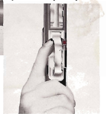
2 To load next shell keep carrier lock button depressed and repeat step 1.
