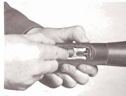
3 To fire, take off safety by pushing button from right to left so that red band appears.
