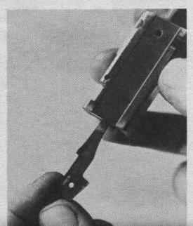
13. Move the firing pin forward to nudge the spring out of its tunnel in the bolt, and remove the spring and the two ball bearings from the extractor recess. Again, take care that the ball bearings aren't lost.
