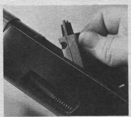
4. Move the bolt toward the rear to clear its forward end from the barrel throat, and tip the front of the bolt upward (the gun is still inverted) until it can be removed from the receiver. Caution: The bolt spring is under tension. Ease it out.
