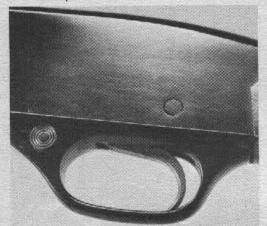
Tip the trigger housing down at the rear, and move it slightly toward the rear to disengage its forward stud from its recess inside the receiver. Remove the trigger group downward.
