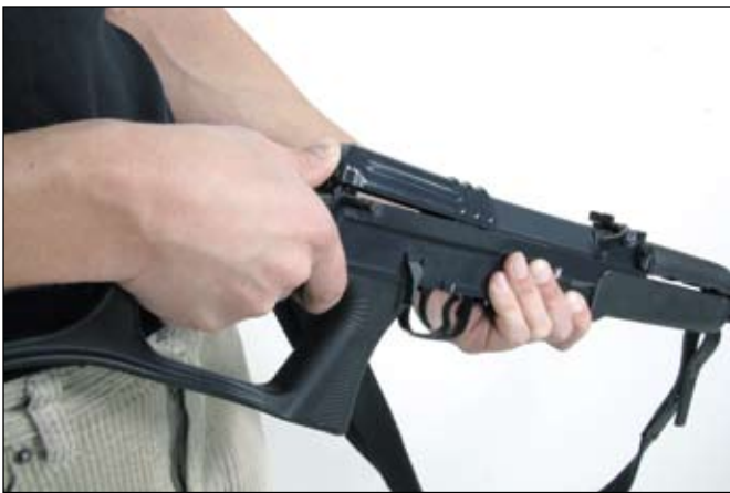
Fig. 28 Removing the return mechanism
