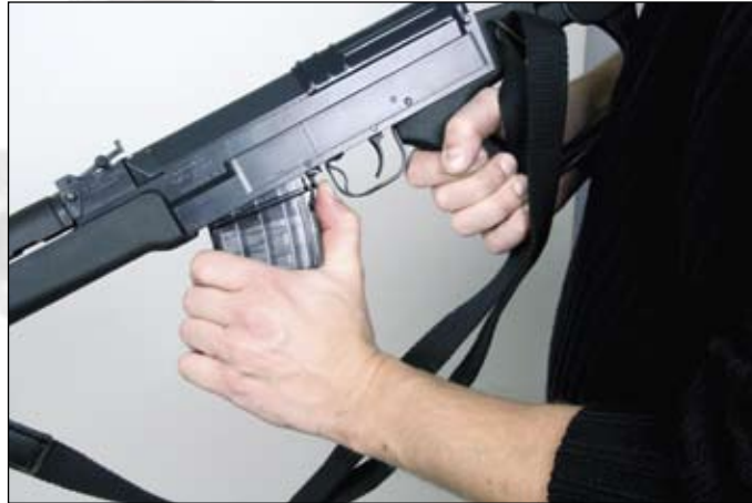
Fig. 27 Taking out the magazine
