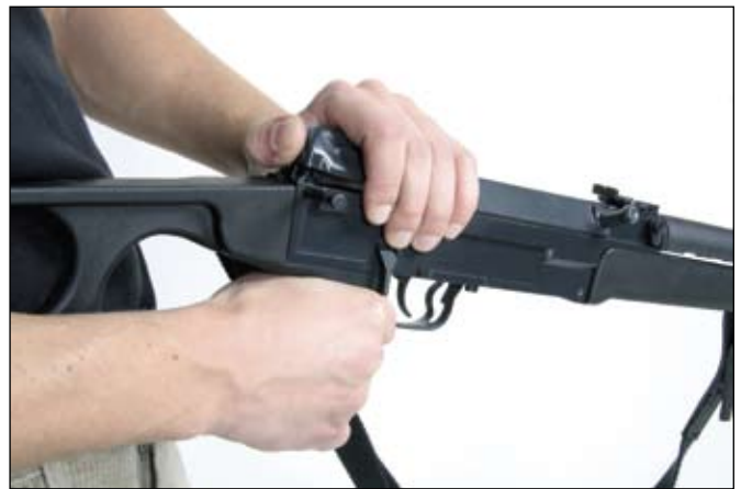
Fig. 29 Removing the return mechanism
