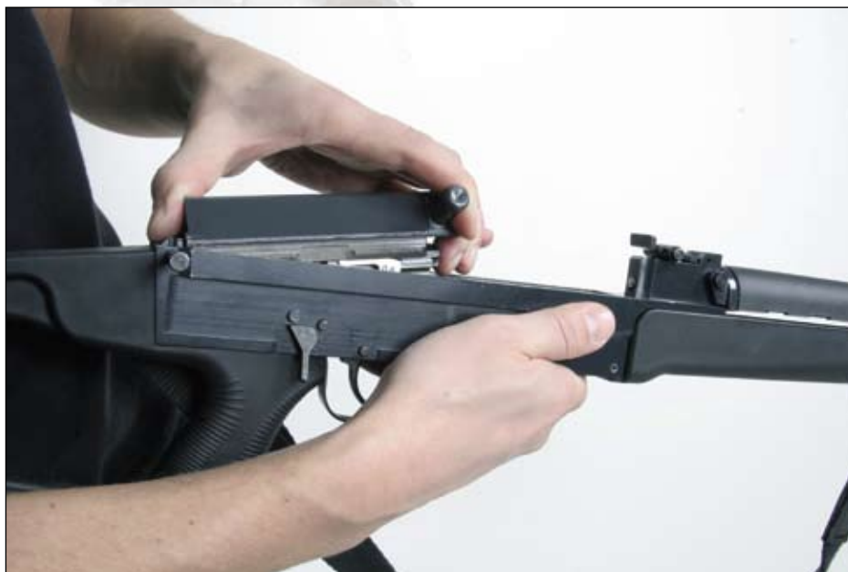
Fig. 30 Taking out the bolt
