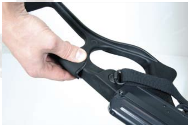
Fig. 32 Attaching the cheek piece
