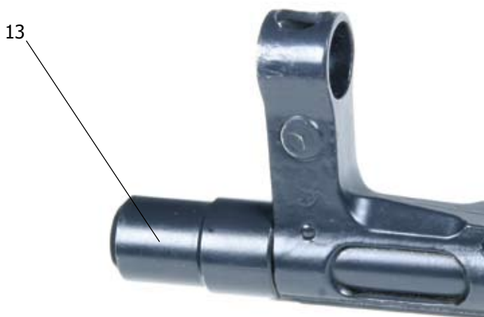
Fig 5. Barrel extension /side view/ 13 - barrel extension
