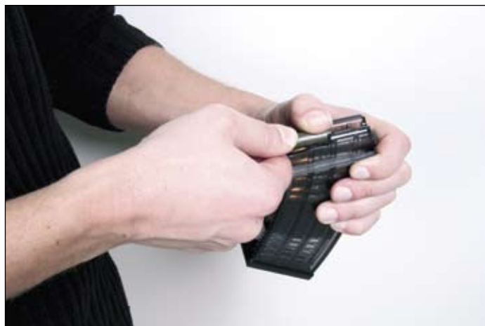
Fig. 24 - Loading the magazine
