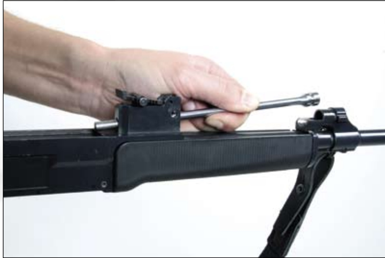
Fig. 31 Removing the piston
