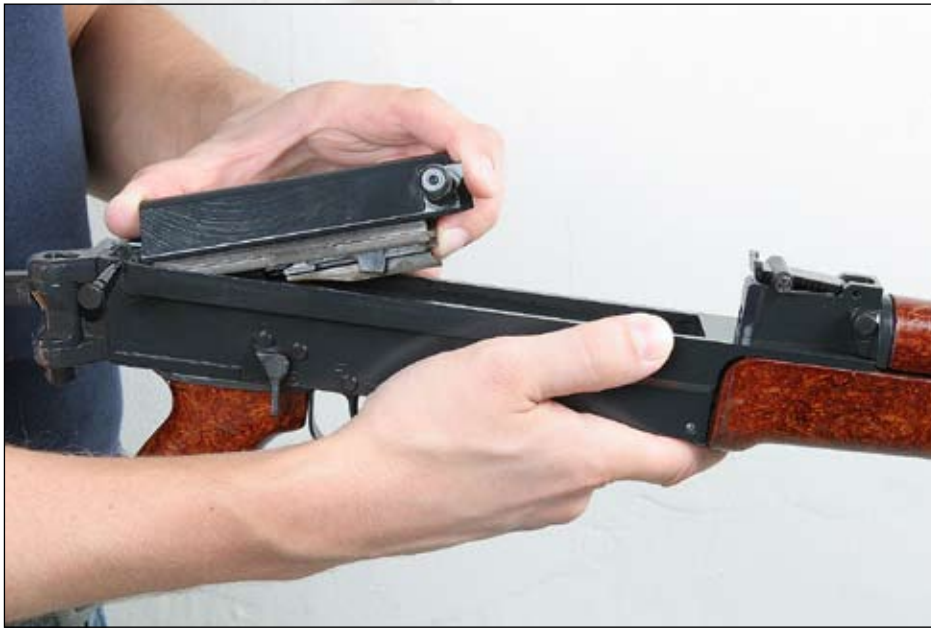
Fig. 30 Taking out the bolt
