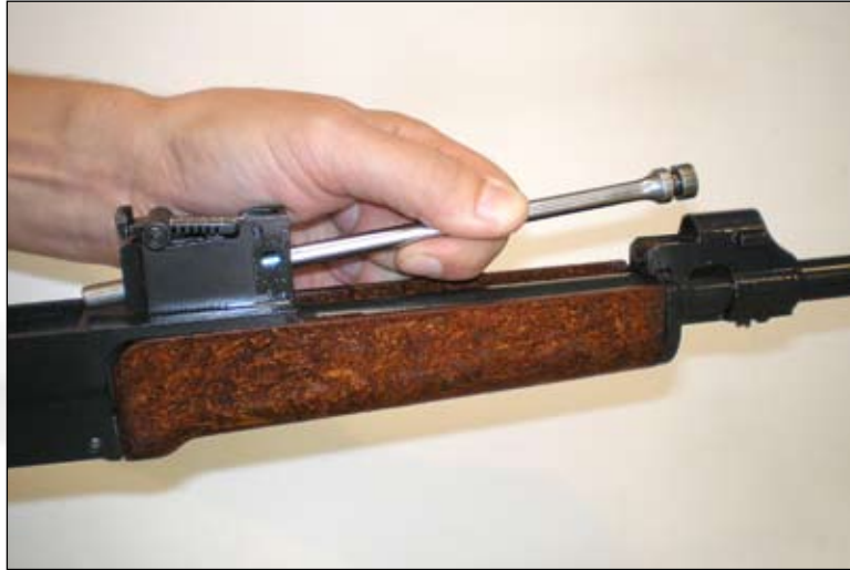
Fig. 31 Removing the piston
