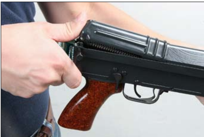
Fig. 28 Removing the return mechanism
