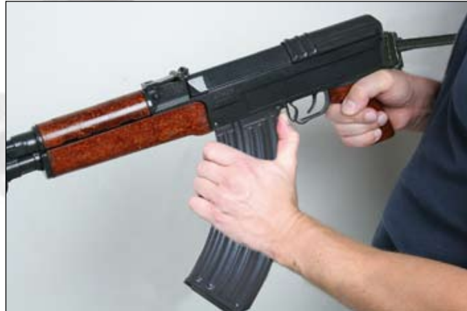
Fig. 27 Taking out the magazine
