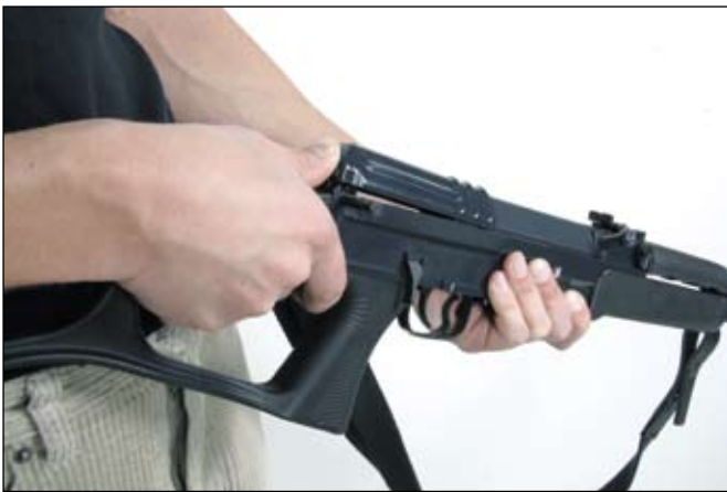
Fig. 28 Removing the return mechanism
