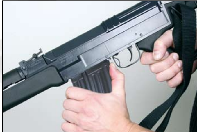
Fig. 27 Taking out the magazine
