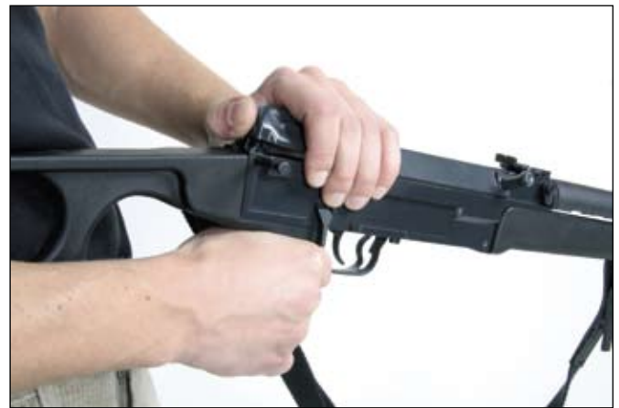
Fig. 29 Removing the return mechanism
