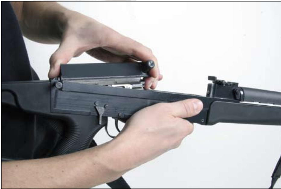
Fig. 30 Taking out the bolt
