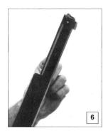
With the follower fully forward, the forward section of the barrel will rotate clockwise. (Photo 6).
