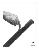
your face and at an angle so that the cartridges slide slowly down the magazine. Capacity is 5 on the 16" Trapper, 6 on the 18" Trapper, 8 on the 22" Carbine and 10 on the 24" 1/4 Rifle.
