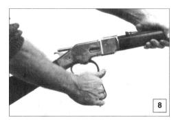
The rifle will now be fully cocked and will fire when the trigger is pulled. If the lever does not go forward, release the loading lever latch by turning the small knob perpendicular to the rifle.
