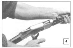
(8) Repeat step 7 until all cartridges have been ejected from the firearm.
