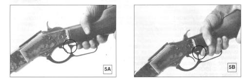
(5) After you have fired the first shot, the next cartridge is loaded by repeating step 3. UNLOADING THE FIREARM
