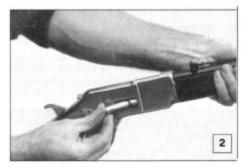
When loading cartridges through the ladle, leave the rim of each cartridge protruding sufficiently to hold the ladle open.
