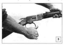
The rifle will now be fully cocked and will fire when the trigger is pulled. If the lever does not go forward, release the loading lever latch by turning the small knob perpendicular to the rifle.
