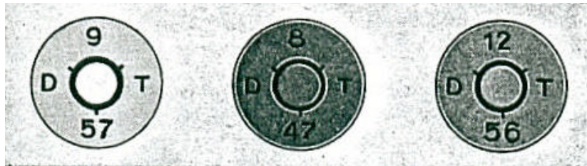
Common Cartridge Armor Piercing Cartridge Tracer Cartridge (No Color) (Purple) (Red) Cartridge Bases Fig. 30
