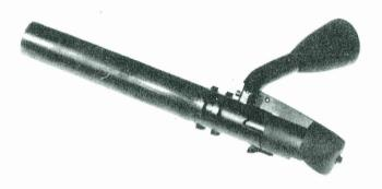
The ergonomic shaped bolt handle allows quick unloading and loading due to the fact that opening angle is only 60°. This feature gives the possibility to mount scopes at a very low mounting height.
