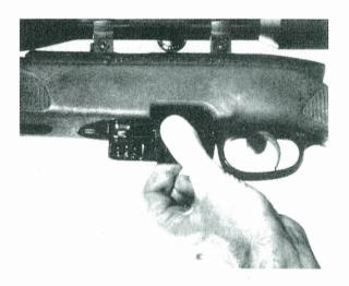
Open the bolt, pull it back completely and close bolt again. By doing so, a cartridge is fed into the chamber.
