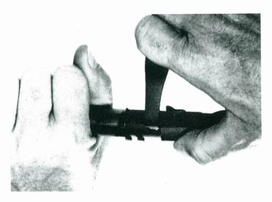
Now the firing pin is cocked and the bolt can be inserted into the receiver. Index finger of left hand pulls trigger and right hand shifts bolt with long end first into receiver. Make sure that firing pin lug faces downwards and safety is on "fire" (red dot visible). Turn bolt handle 60° clockwise whilst pulling the trigger. The firing pin is now decocked; this is indicated by the red end of the firing pin which has now disappeared in the slide cap.
