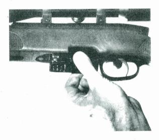
Place head of cartridge where the magazine allows inserting and slide it back to magazine cover. The magazine can hould 5 rounds.
