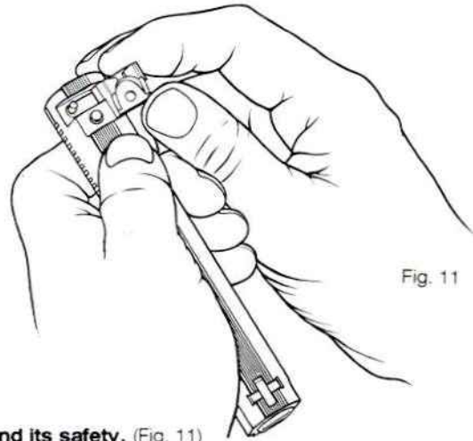
Access to the firing pin and its safety. (Fig. 11)
