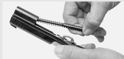
Fig. 4 Remove the recoil / buffer spring guide rod
