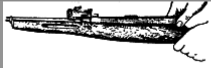
Figure 9: Separating the barrel with receiver from the stock
