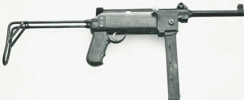
Machine pistol Neuhausen MP 48 with magazine and stock out
