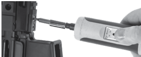
FIG 52 TIGHTENING OF RAIL CLAMP SCREWS
