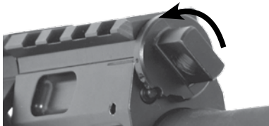
FIG 11 GAS VALVE ON SUPPRESSED MODE (ACTION WILL CYCLE)
