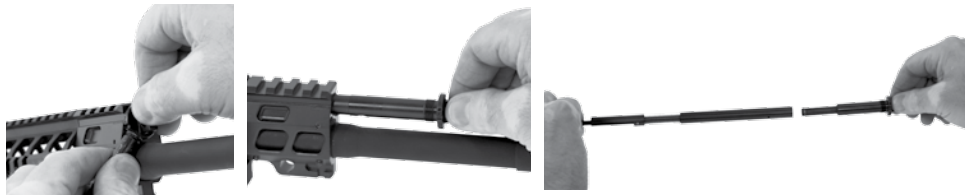
FIG 30 PICTURE OF THE GAS VALVE BEING REMOVED
