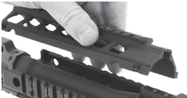
FIG 50 RE-INSTALLATION OF LOWER RAIL SECTION
