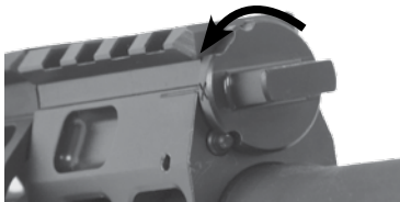
FIG 12 GAS VALVE ON P4 POSITION, SUPPRESSED MODE (THE ACTION WILL NOT CYCLE)
