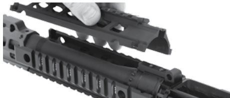
FIG 34 REMOVAL OF THE LOWER RAIL SECTION
