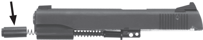
Fig. 2: Removal of recoil spring plug and recoil spring
