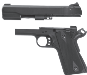
Fig. 4: Slide completely removed
